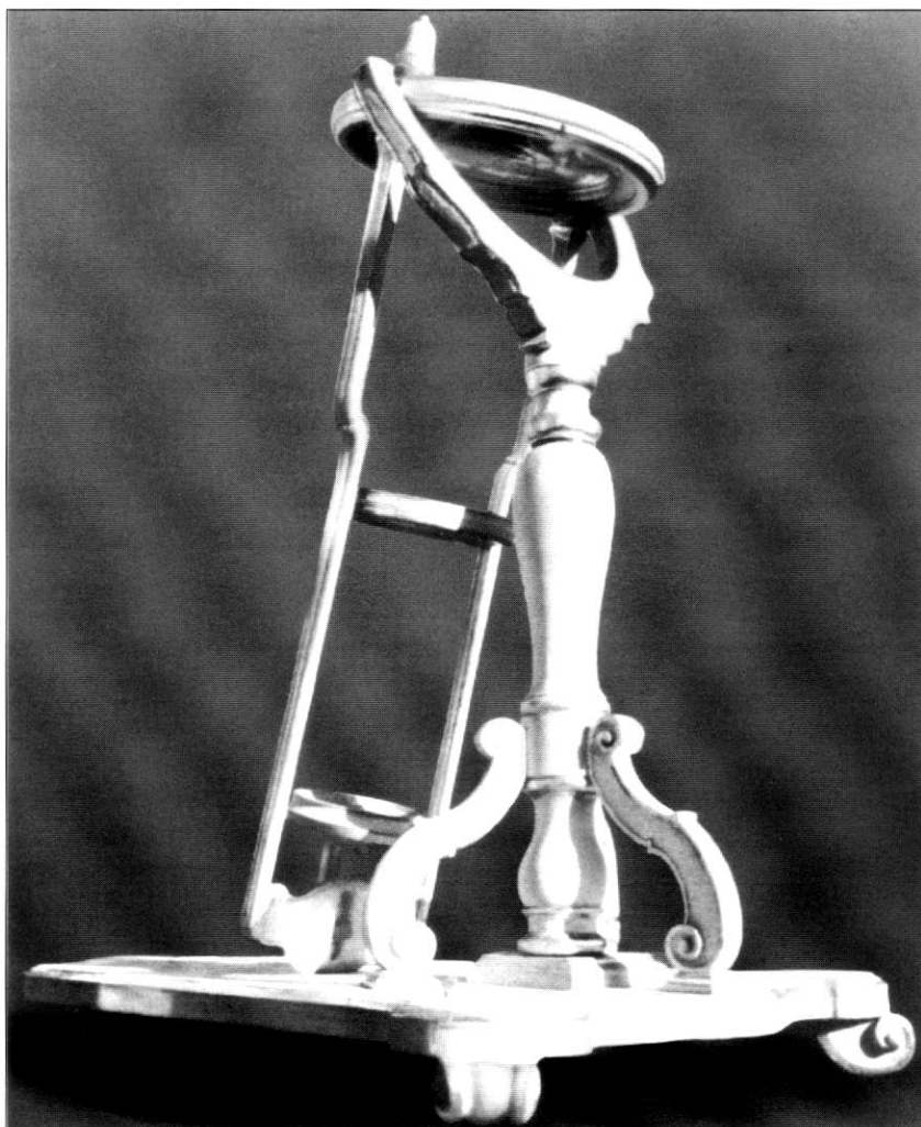
Fig. 5. "Burning glass" solar furnace of the type used in Meissen porcelain research.
