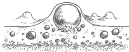
Pox, > 400 \mu\text{m} , bulges on surface, locally or spread over product, underlying bubbles are bigger than 100 \mu\text{m}
