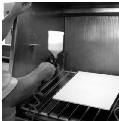
Figure 1. Application of additive suspensions on porcelain stoneware pieces.
