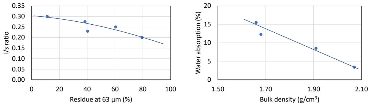
**Figure 1.** Evolution of the I/s ratio with waste particle size (left) and of water absorption with bulk density (right)
