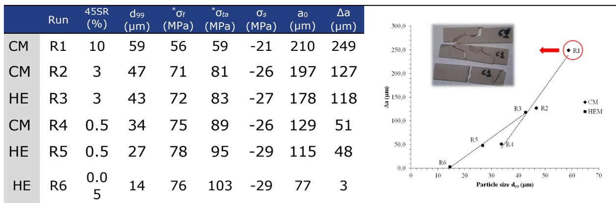
**Table 1.** Results of particle size (45SR,  $d_{99}$ ), bending strength ( $\sigma_f$  slow and  $\sigma_{ta}$  high cooling rate), Macroscopic residual stress ( $\sigma_s$ ), flaw size ( $a_0$ ), increased flaw size ( $\Delta a$ )
