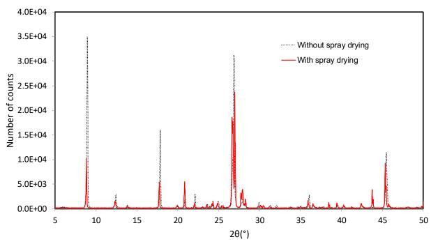
**Figure 3** Diffractogram of a clay sample without and with the spray-drying process in the unit developed at ITC
