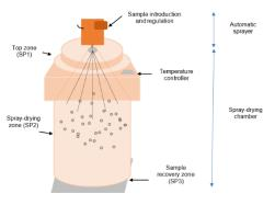
*Figure 2 Micro spray-drying unit developed at ITC*
