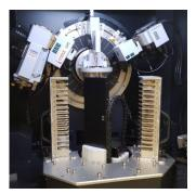
Fig. 1 X-ray diffractometer
