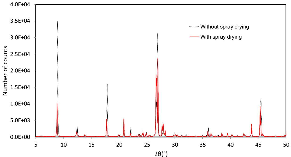
**Figure 3** Diffractogram of a clay sample without and with the spray-drying process in the unit developed at ITC
