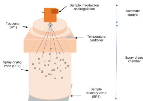
**Figure 2** Micro spray-drying unit developed at ITC
