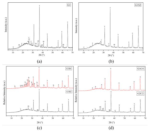
*Figure 1. XRD* patterns of samples a) G1 glaze b) G1S2 glaze c) G1B2 and G1B4 glaze d) G1C2 and G1C4 glazes (c: cordierite, m: mullite, s:spinel, r strontium aluminium silicate, h:celsian, a:anorthite)
