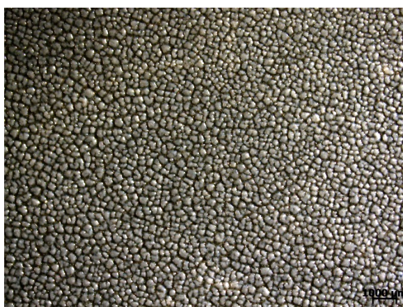
Figure 2. Stereo microscope image of granilla-like effect. The amount of applied material is 60 g solid/m 2 .
