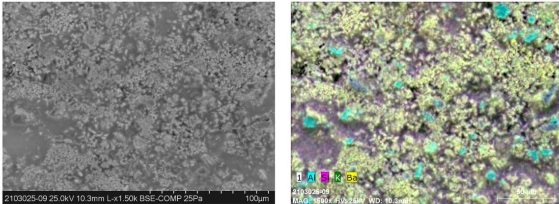
**Figure 3.** Micrograph of the surface of glaze PF-026/7 (left) and mapping (right).
