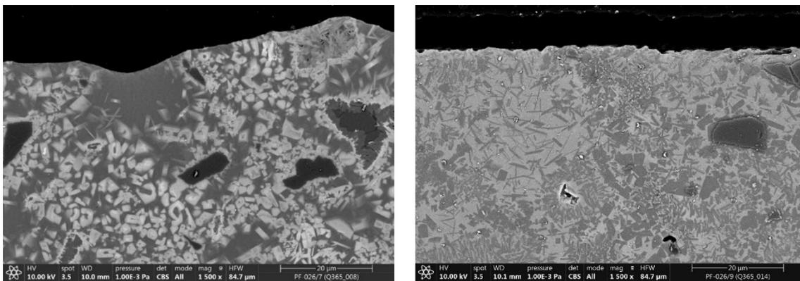
**Figure 2.** Micrograph of the cross-section of glaze PF-026/7 (left) and PF-026/9 (right).
