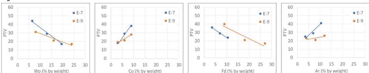
**Figure 7.** Influence of the variation of each raw material on slip resistance.
