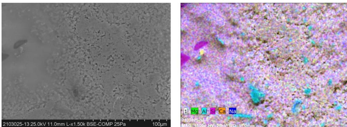
**Figure 4.** Micrograph of the surface of glaze PF-026/9 (left) and mapping (right).
