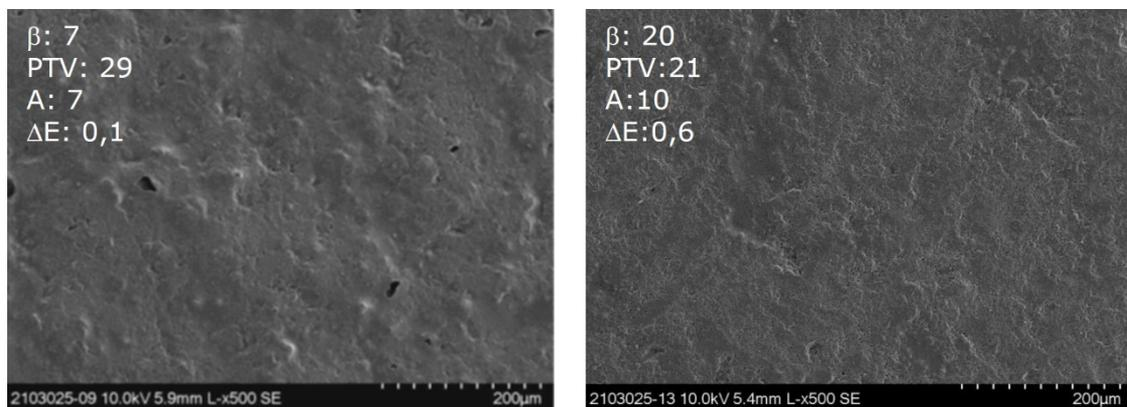
**Figure 1.** Micrographs of the surface of glaze PF-026/7 (left) and PF-026/9 (right).
