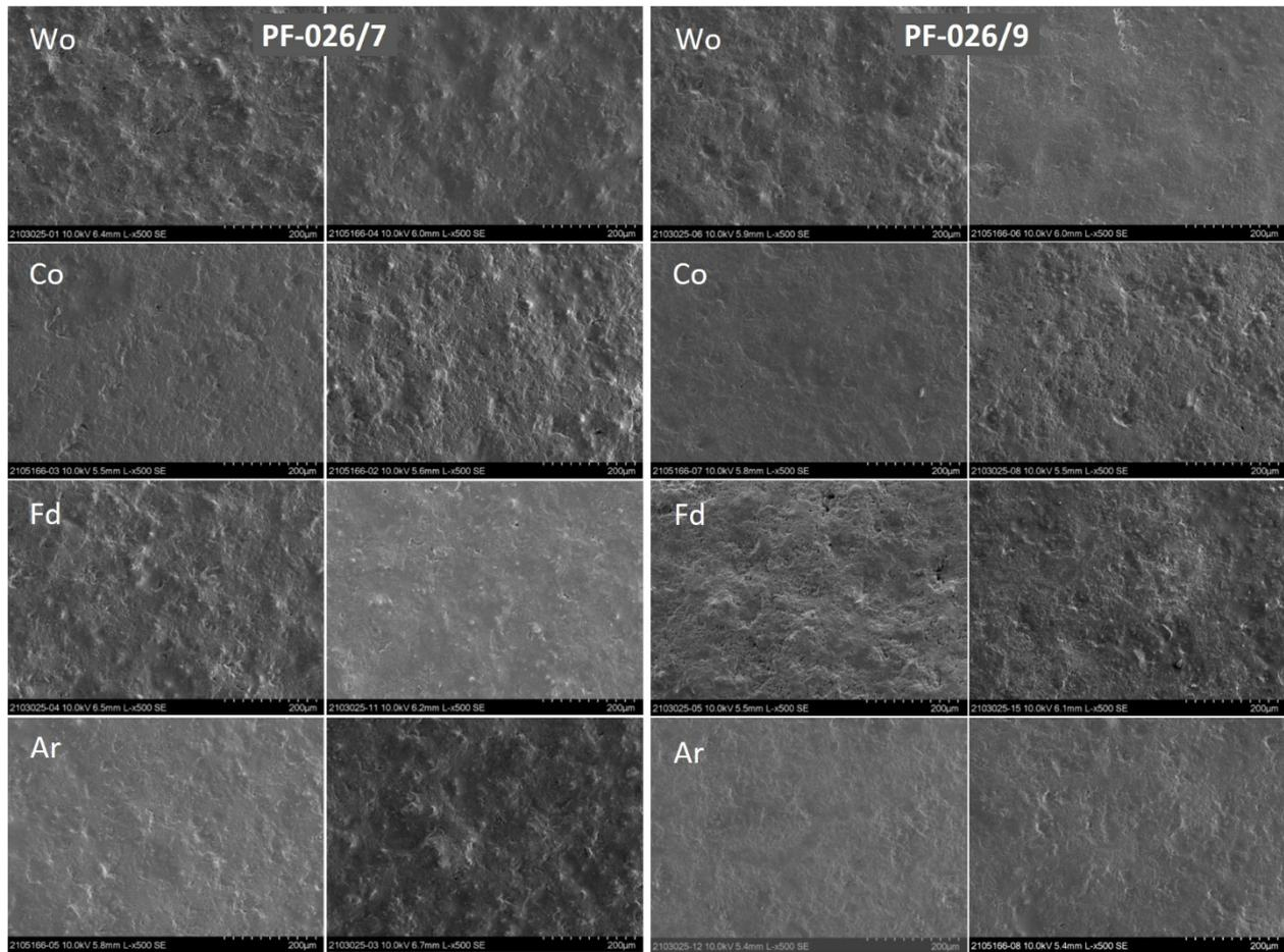
**Figure 5.** Micrographs of glaze PF-026/7 and PF-026/9 with a different content (left: decrease and right: increase) of each raw material.
