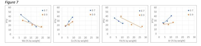
Figure 7. Influence of the variation of each raw material on slip resistance.
