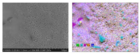
Figure 4. Micrograph of the surface of glaze PF-026/9 (left) and mapping (right).
