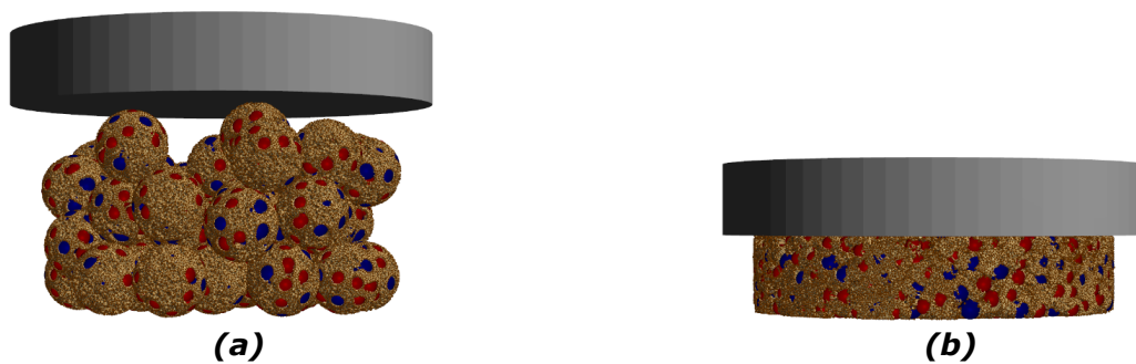
Fig. 8 Simulation scene (a) Before compaction (b) After compaction reaching 60% strain deformation
