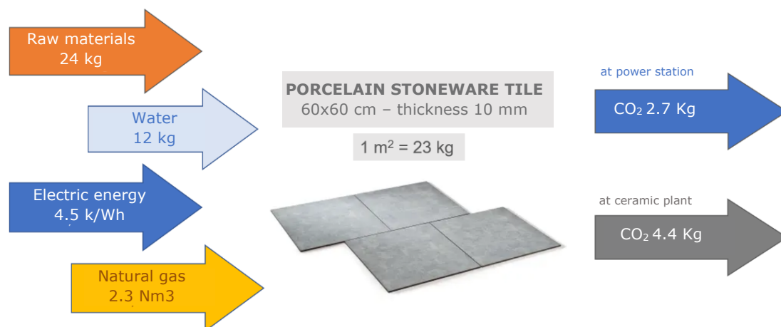
Fig. 4 – Mass and energy balance in the ceramic production process
