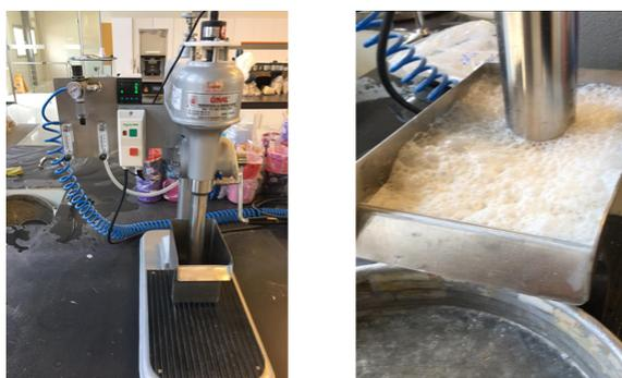
**Figure 1:** Flotation cell where flotation experiments are carried out.
