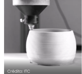
Figure 1 3D printing of a ceramic piece.
