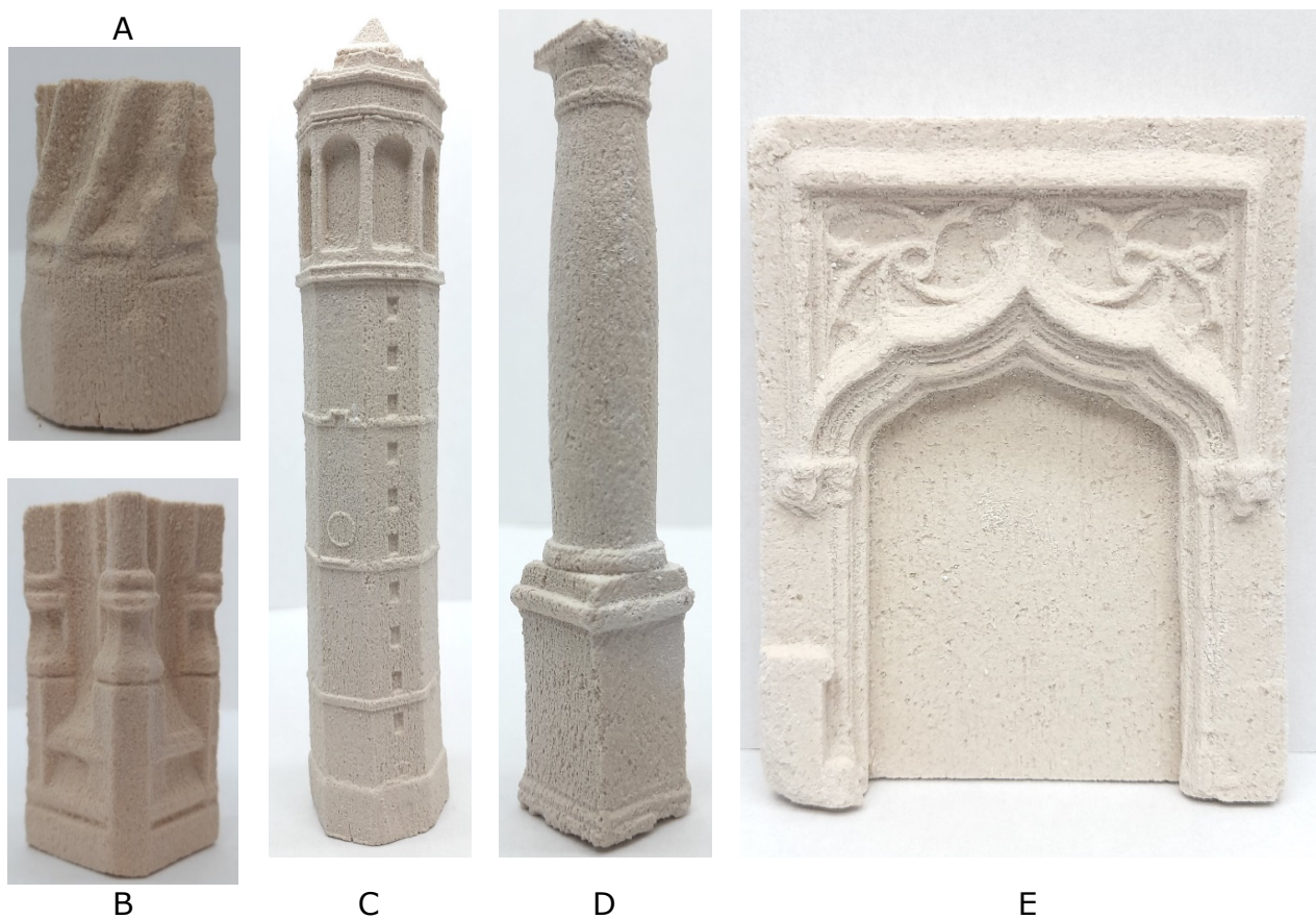
Figure 18 Pieces made by BJ with ceramic material: A) Base of a column at the Valencia Central Market (Lonja). B) Detail of a window at the Monastery of Cotalba, C) Bell tower of Castellón, D) Column at the Dominican cloisters, E) Portal on the main floor of the Consulate of the Sea.
