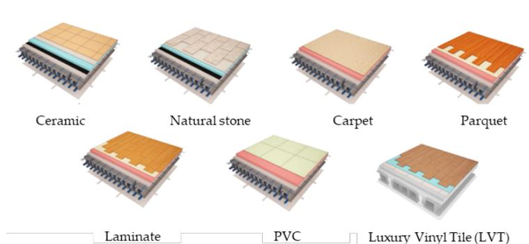
**Figure 1.** The different ceramic solutions for flooring considered in present study.
