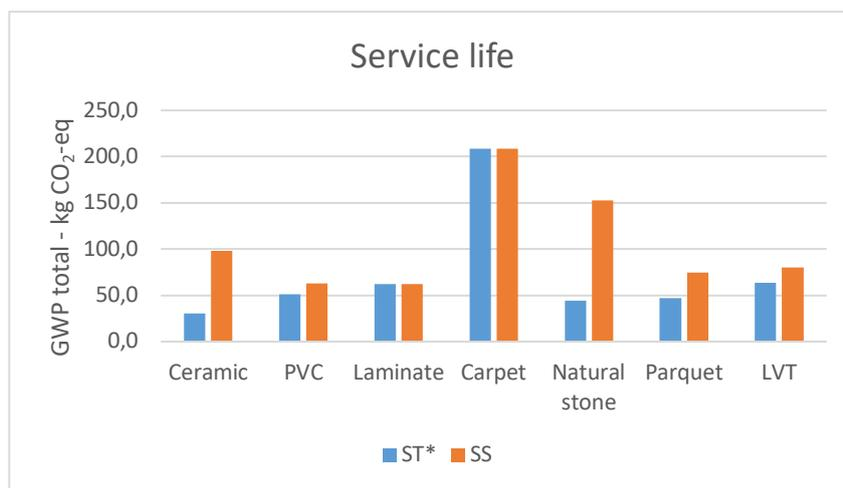
**Figure 4.** Lifecycle climate impact (GWP total) of the assessed floor systems. Comparison between the two scenarios for service life where ST represents the technical service life (see Table 2; column MSL) and SS the scenario where all floor systems were assessed with the same service life (15 years). The default scenario is indicated with \*.
