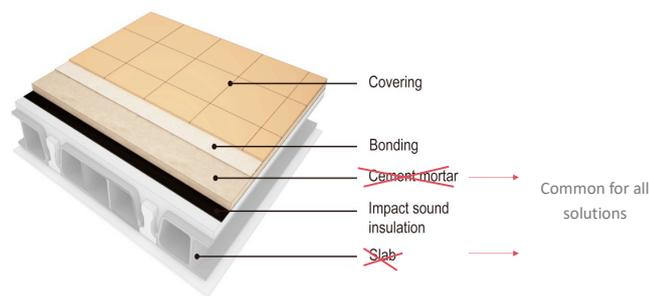
**Figure 2.** Detailed of the construction system considered in the present study
