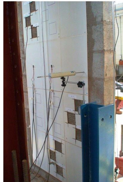
**Figure 3** – Horizontal transducer as installed.
