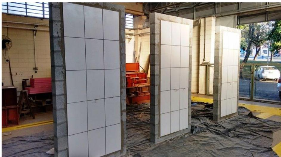
**Figure 1** – Wall specimens built in the laboratory for the experimental study.
