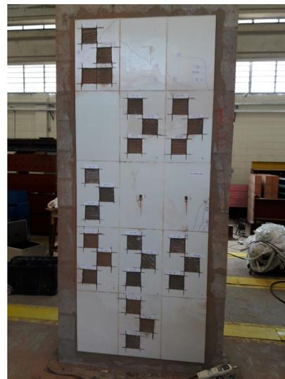
**Figure 8** – Wall specimen after the compression test procedure.
