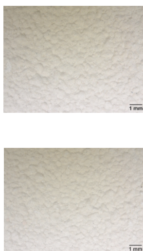
Figure 8. Surface micrography of the pressed tiles MIX (above) and STD (below).
