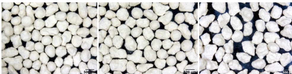
Figure 5. Micrographs of the samples 500-710\mu\text{m} . STD (left), MIX (centre) and SCRAP (right).
