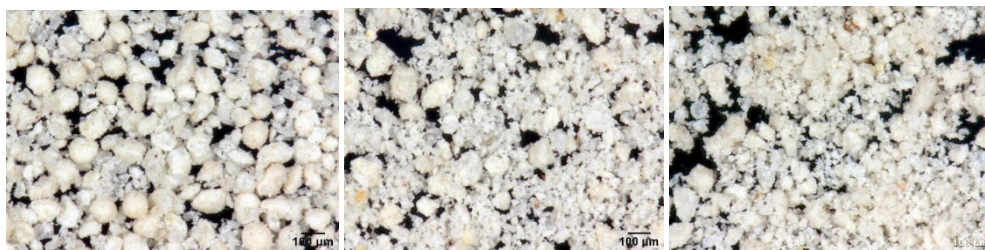
Figure 4. Micrographs of the samples <125\mu\text{m} . STD (left), MIX (centre) and SCRAP (right).
