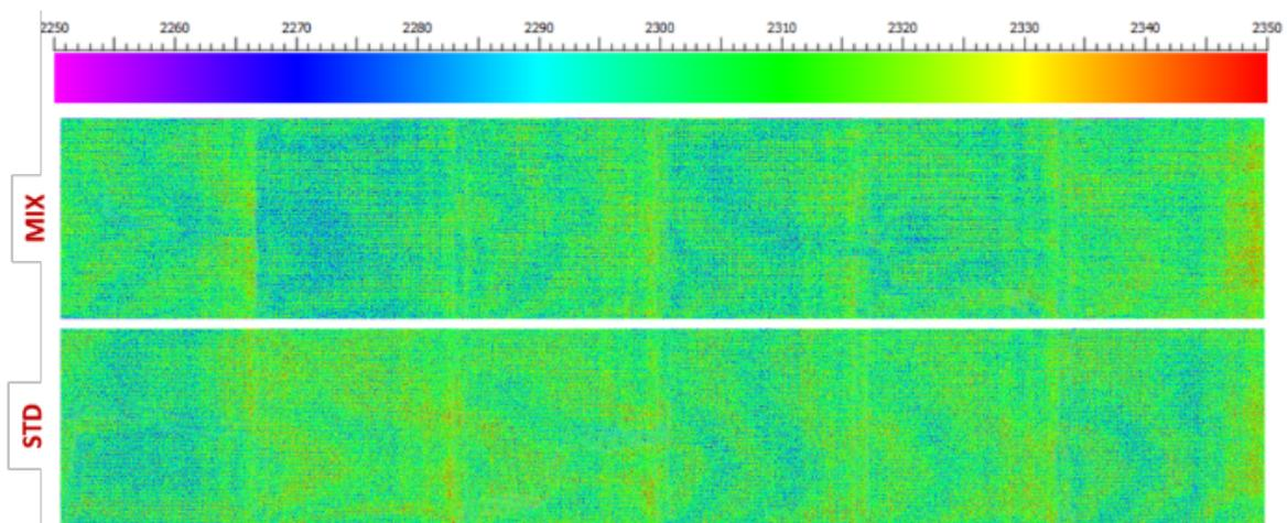
**Figure 12.** Fired density (kg/m<sup>3</sup>) distribution of six 900 mm x 900 mm tiles obtained from green cutting of a big slab.
