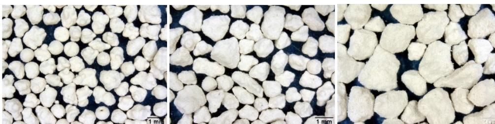
**Figure 6.** Micrographs of the samples >710µm. STD (left), MIX (centre) and SCRAP (right).
