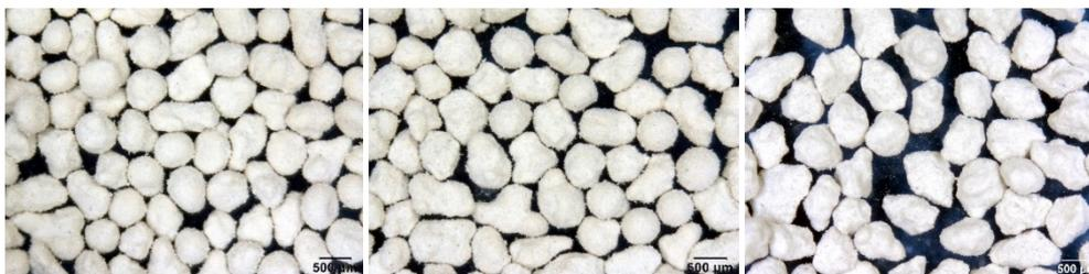
**Figure 5.** Micrographs of the samples 500-710 µm. STD (left), MIX (centre) and SCRAP (right).
