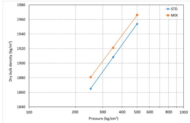
**Figure 7.** Evolution of dry bulk density with pressing pressure.
