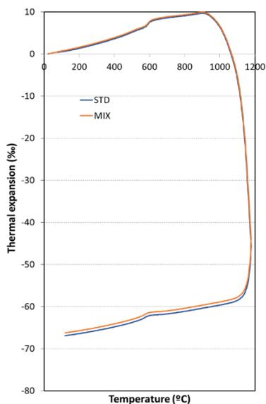
**Figure 9.** Expansion-shrinkage curves for both tested materials.
