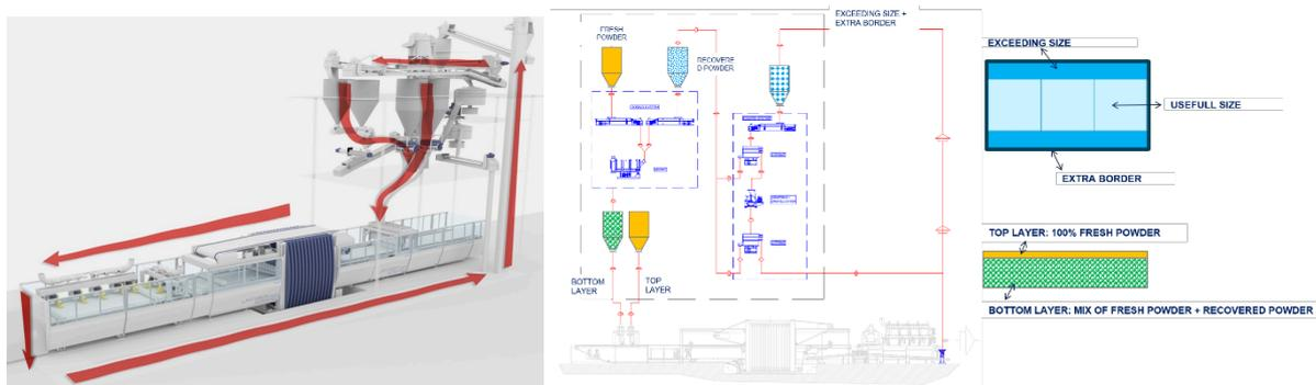
**Figure 2.** General powder flows in the developed scrap recovering system (left) and detail of the different powder layers constituting the product (right).
