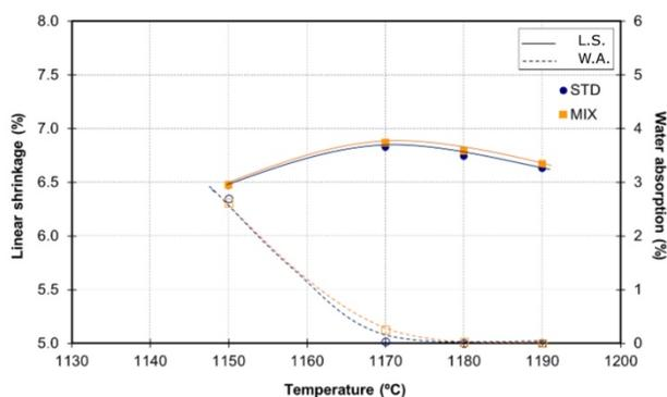
**Figure 10.** Linear shrinkage (L.S.) and water absorption (W.A.) with temperature. Vitrification diagram.
