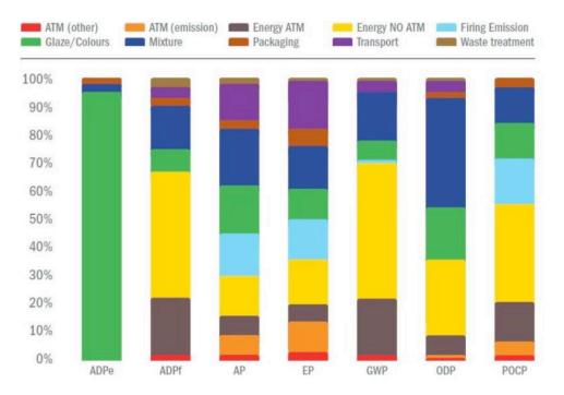
**Figure 7:** Impacts due to Italian ceramic tile manufacturing. ADPE = abiotic depletion potential for non-fossil resources; ADPF = abiotic depletion potential for fossil resources; AP = acidification potential of land and water; EP = eutrophication potential; GWP = global warming potential; OPD = depletion potential of the stratospheric ozone layer; POCP = formation potential of tropospheric ozone photochemical oxidants.
