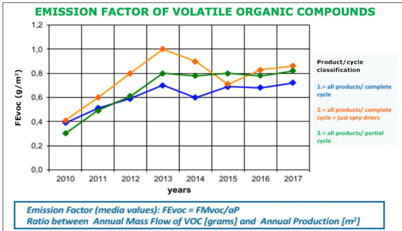
**Figure 3:** VOC emission factor - annual average values considering the classification on products and process.
