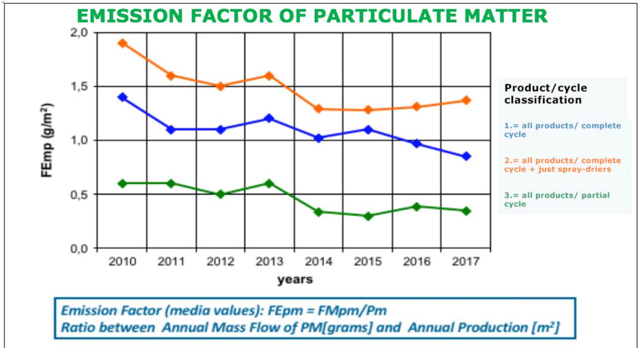
**Figure 1:** Emission Factor ( $FE_{MP}$ ) of Particulate Matter from years 2010 to 2017 considering the classification on products and processes.
