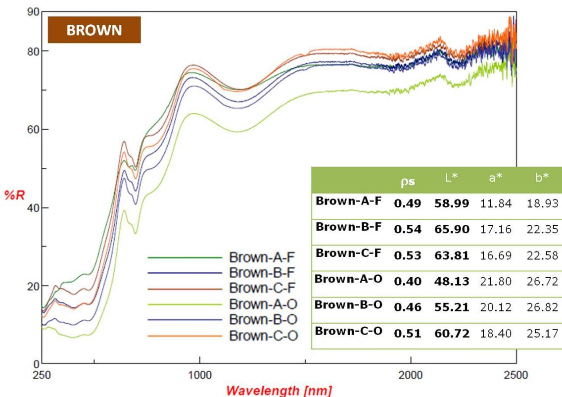
**Figure 4:** Solar reflectance curves (reflectance,  $R$ , versus spectral wavelength), solar reflectance values ( $\rho_s$ ) and colorimetric coordinates ( $L^*$ ,  $a^*$ ,  $b^*$ ) of the brown samples.
