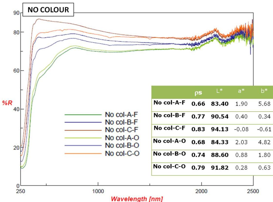
Figure 7: Solar reflectance curves (reflectance,  $R$ , versus spectral wavelength), solar reflectance values ( $\rho_s$ ) and colorimetric coordinates ( $L^*$ ,  $a^*$ ,  $b^*$ ) of the no colour samples.
