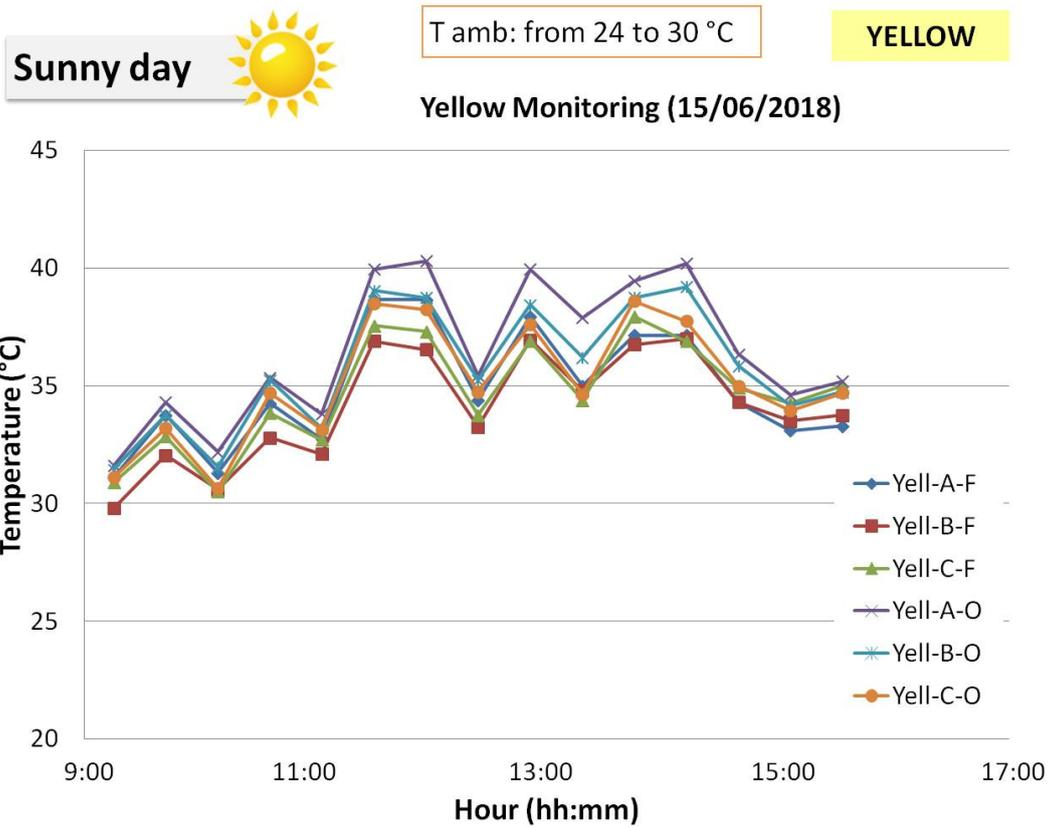
**Figure 9:** Surface temperature curves of the yellow samples, on a sunny day during monitoring.
