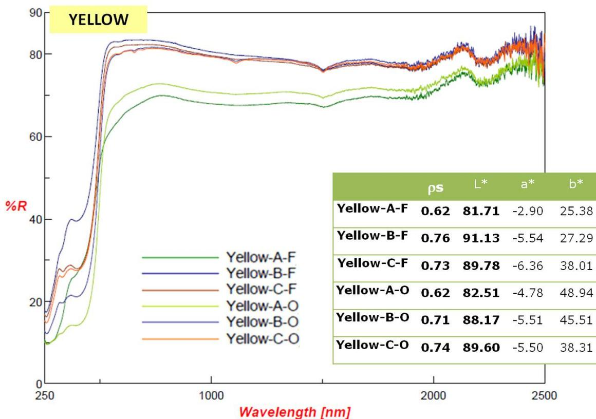
Figure 6: Solar reflectance curves (reflectance,  $R$ , versus spectral wavelength), solar reflectance values ( $\rho_s$ ) and colorimetric coordinates ( $L^*$ ,  $a^*$ ,  $b^*$ ) of the yellow samples.
