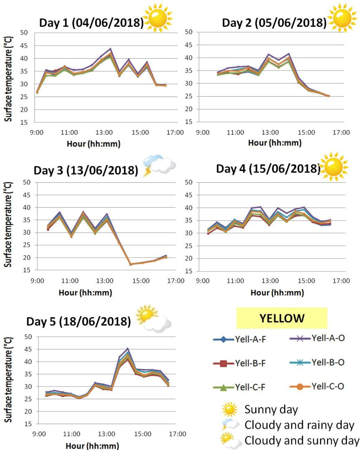
**Figure 8:** Surface temperature curves of the yellow samples during 5 days of monitoring.
