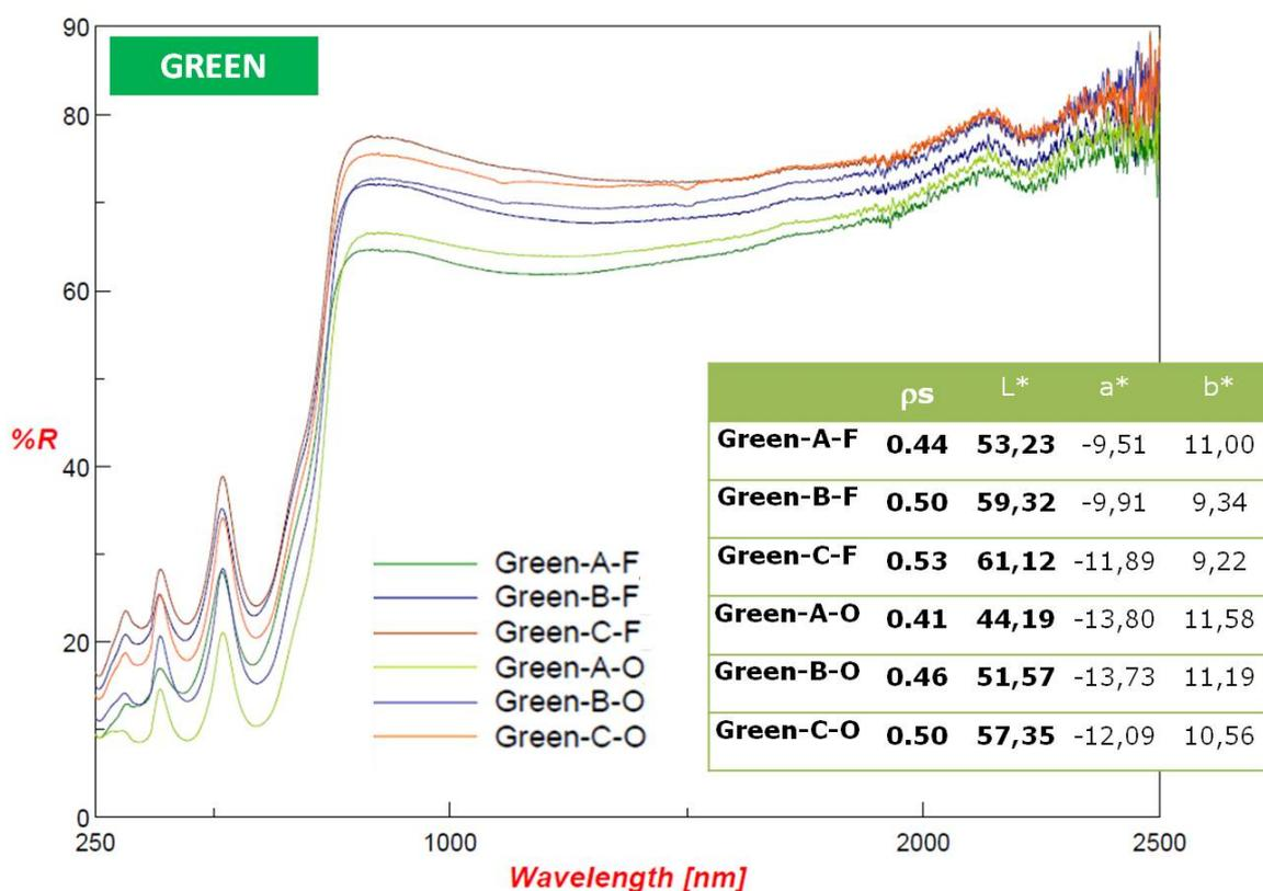
**Figure 5:** Solar reflectance curves (reflectance,  $R$ , versus spectral wavelength), solar reflectance values ( $\rho_s$ ) and colorimetric coordinates ( $L^*$ ,  $a^*$ ,  $b^*$ ) of the green samples.
