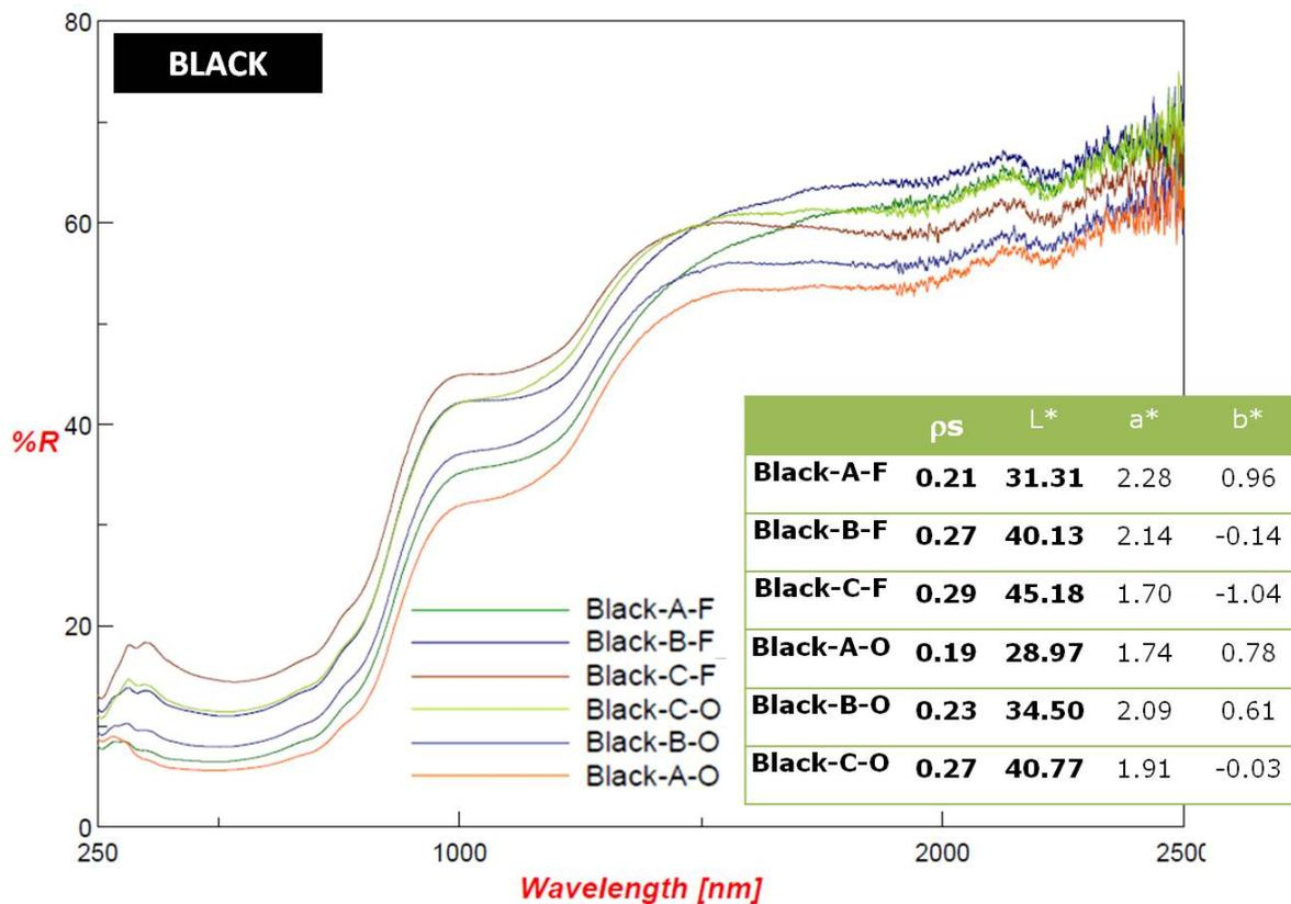
Figure 2: Solar reflectance curves (reflectance,  $R$ , versus spectral wavelength), solar reflectance values ( $\rho_s$ ) and colorimetric coordinates ( $L^*$ ,  $a^*$ ,  $b^*$ ) of the black samples.
