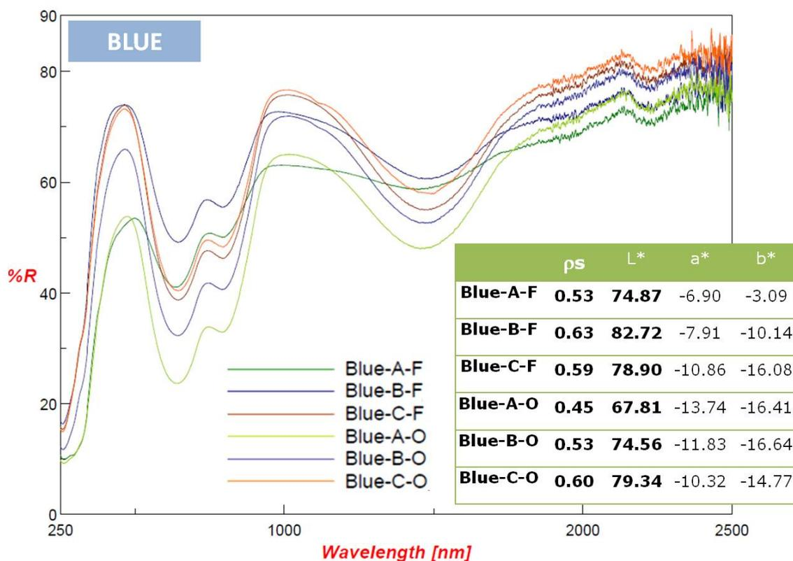
Figure 3: Solar reflectance curves (reflectance,  $R$ , versus spectral wavelength), solar reflectance values ( $\rho_s$ ) and colorimetric coordinates ( $L^*$ ,  $a^*$ ,  $b^*$ ) of the blue samples.
