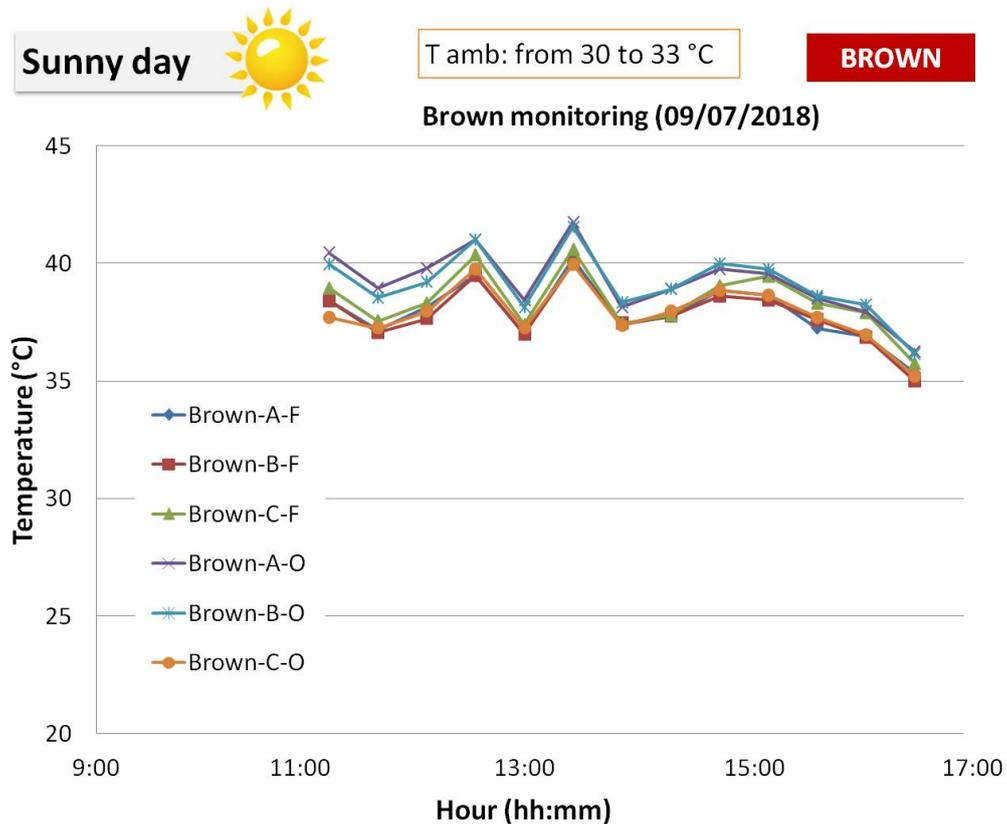
**Figure 10:** Surface temperature curves of the brown samples, on a sunny day during monitoring.
