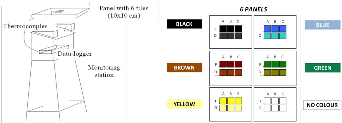
**Figure 1:** Scheme of the monitoring station (left) and panels with the samples (right).
