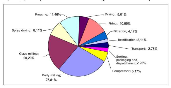
**Figure 1.** Distribution of power consumption in a ceramic tile manufacturing company using wet milling in Brazil (obtained from data provided in [4])
