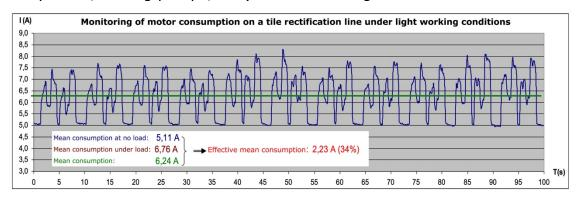
**Figure 4.** Monitoring of consumption by a motor on a ceramic tile rectification line working under light/medium load conditions, where consumption at no load represents 75.5% of consumption under load and effective mean consumption is 34%.
