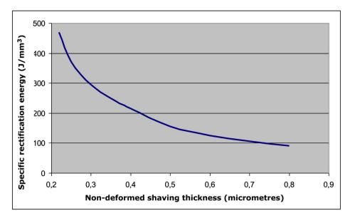
**Figure 3**. Influence of maximum thickness of removed shaving,  $h_{max}$ , on the value of specific machining energy in the case of an alloy steel
