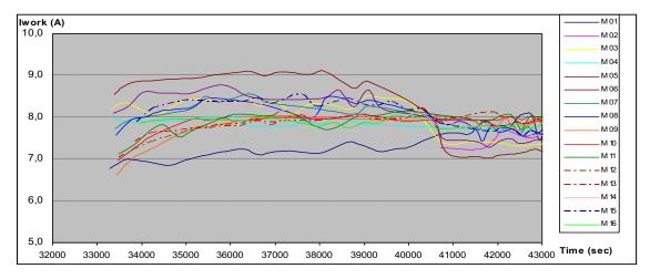
**Figure 5**. Motor consumption monitoring system for a 16-head ceramic tile rectification line, showing the process to adjust the heads to ensure all of them work at the target consumption level of 7.8 A.
