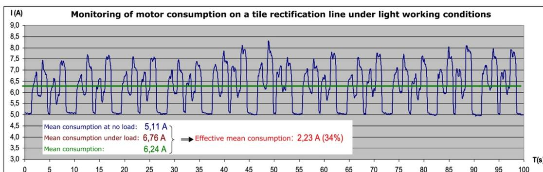
**Figure 4.** Monitoring of consumption by a motor on a ceramic tile rectification line working under light/medium load conditions, where consumption at no load represents 75.5% of consumption under load and effective mean consumption is 34%.
