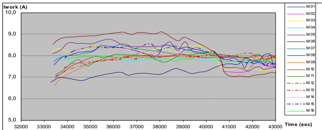
**Figure 5.** Motor consumption monitoring system for a 16-head ceramic tile rectification line, showing the process to adjust the heads to ensure all of them work at the target consumption level of 7.8 A.
