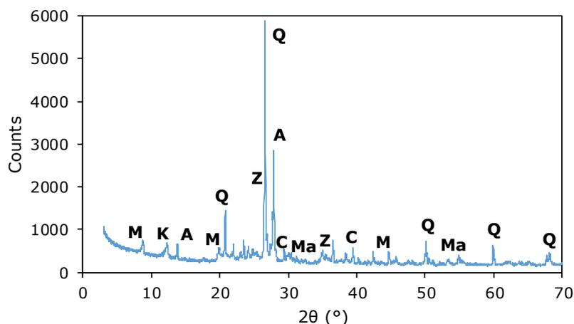
**Figure 1.** XRD pattern of the ceramic sludge (A: Albite, C: Calcite, K: Kaolinite, M: Muscovite, Ma: Magnesite, Q: Quartz, Z: Zircon)
