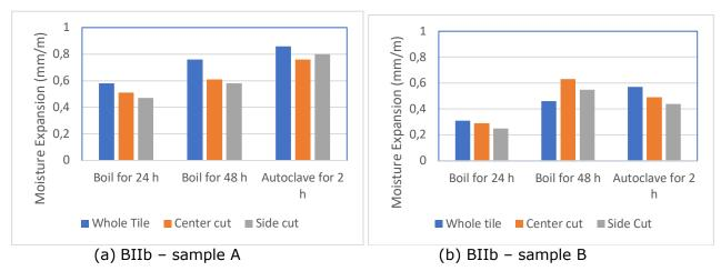
**Figure 1.** Comparison of moisture expansion values as a function of cutting and hydration type: (a) BIIb - sample A and (b) BIIb - sample B.
