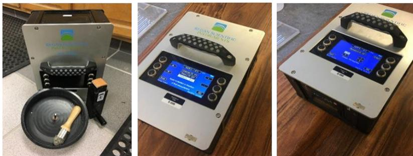
**Figure 5:** ANSI A326.3 equipment used and testing (left to right): BOT 3000E/sensor conditioning wheel/SBR sensor, BOT prior to making a measurement, BOT after making a measurement
