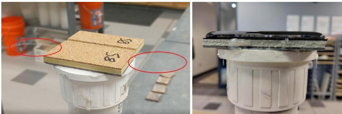
**Figure 4:** Water penetrating the seam and exiting from the edges (left), and water penetrating the seam and leaking onto the back of the sample (right)
