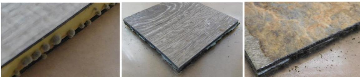
**Figure 6:** Examples of PBM test specimens which supported mold growth
