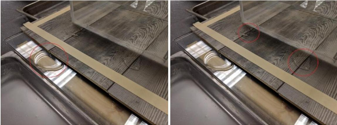
**Figure 3:** Water penetration into the seams and exiting at the edge of the assembly (left), and water penetration into the seams and exiting atop the assembly outside the sealed containment box (right)
