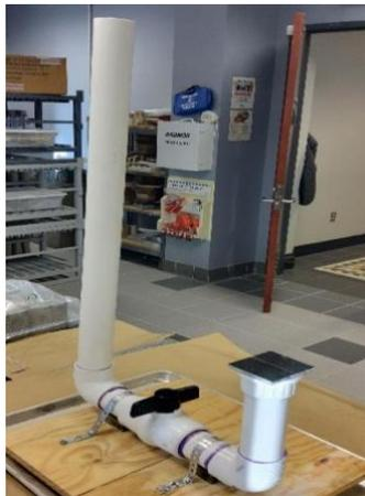
**Figure 2:** Constructed test assembly, per ASTM D4068
