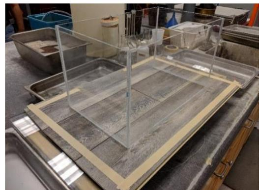
**Figure 1:** Orientation of box-frame in relation to floor covering seams (seams represented by dotted lines) and box-frame installed atop floor covering test specimen
