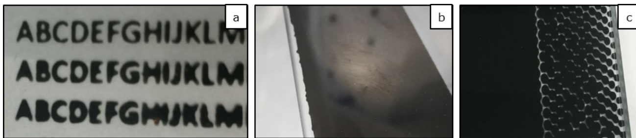
Fig.5: Spread defect for images printed on glass. a) Letters, b) full shade, c) fade out dot area.
