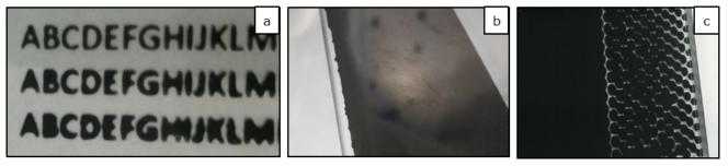
*Fig.5:* Spread defect for images printed on glass. a) Letters, b) full shade, c) fade out dot area.
