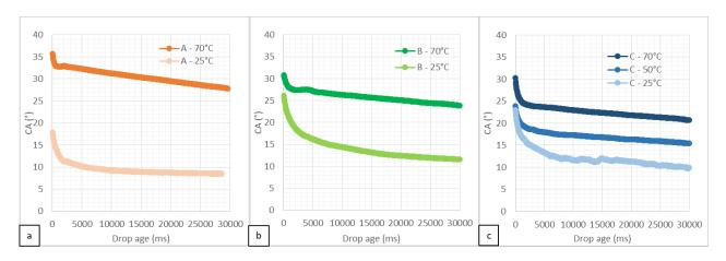
**Fig.4:** Contact angle measurements for three different ink samples at various substrate temperatures as a function of drop age: a) ink A with substrate at 25 and 70°C, b) ink B with substrate at 25 and 70°C, c) ink C with substrate at 25, 50 and 70°C.
