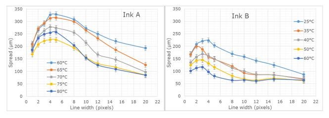
*Fig.9:* Measure of spread for ink A and B at various glass temperatures and increasing line width.
