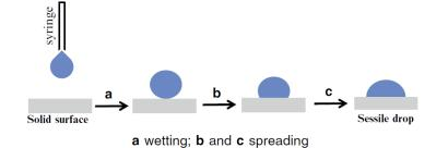
**Fig.2:** Schematic showing the main phases of static contact angle measurement with the sessile drop technique: the drop is ejected from a syringe, lands on the surface and spreads.
