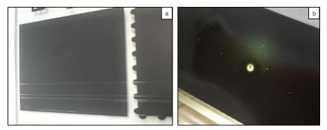
*Fig.6:* a) Missing nozzle defect and b) a "hole" defect in a full shade printed on glass.
