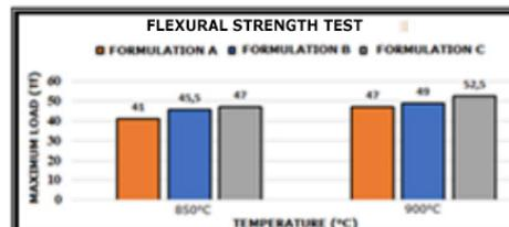
Figure 8 - Flexural strength test in the formulations.
