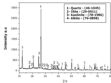
**Figure 3** - X-ray diffraction of kaolin residue.
