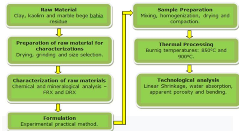
**Figure 1** - Flow chart for the production of ceramic tiles with kaolin residue and Bahia beige marble.
