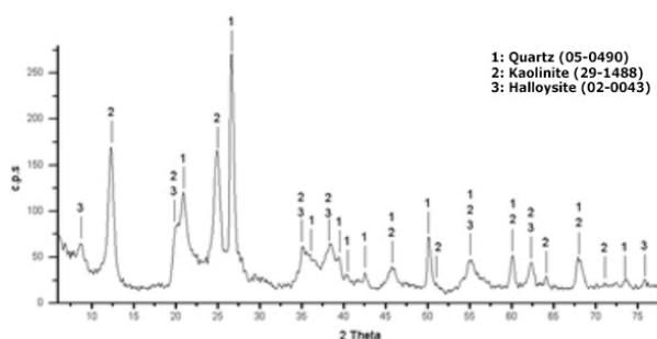
**Figure 2** - X-ray diffraction of clay in nature.
