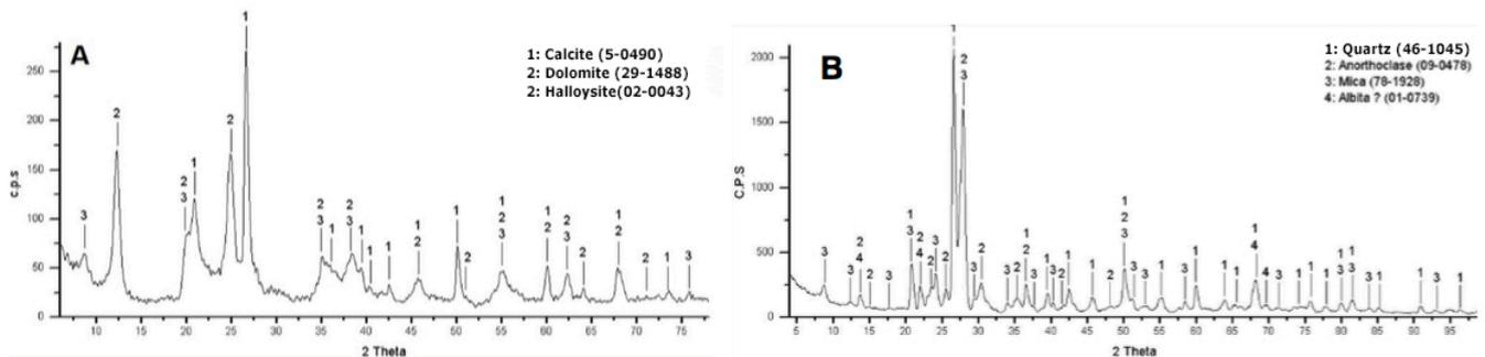
Figure 1: X-ray diffraction of (A) clay and (B) mineral residue.
