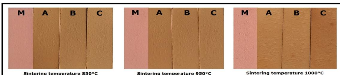
Figure 2: Photos of the test specimens of the formulations studied at a) 850°C, b) 950°C and c) 1000°C, with a heating rate of 10°C / min, for 1 hour.
