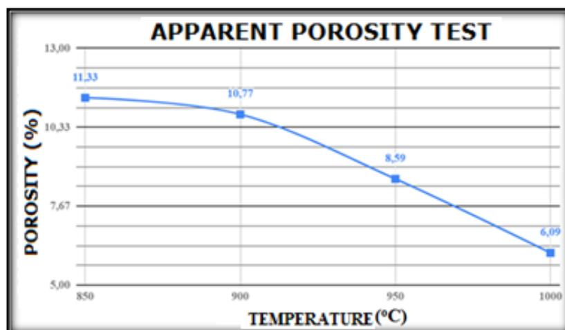
**Figure 6** – Apparent porosity graph in the formulations.
