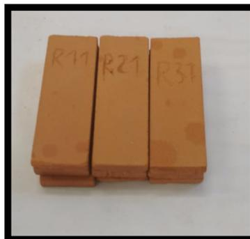
**Figure 8** – Samples fired at 850, 900 and 1000°C.
