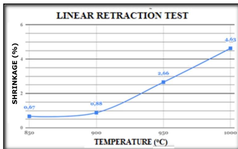
**Figure 4** - Linear shrinkage graph of samples at different firing temperatures.
