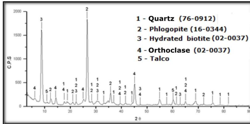
**Figure 3** - Diffractogram of the mineral residue.
