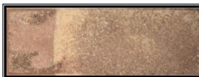
**Figure 10** – Engobed sample with 100% mineral residue fired at 1000°C.
