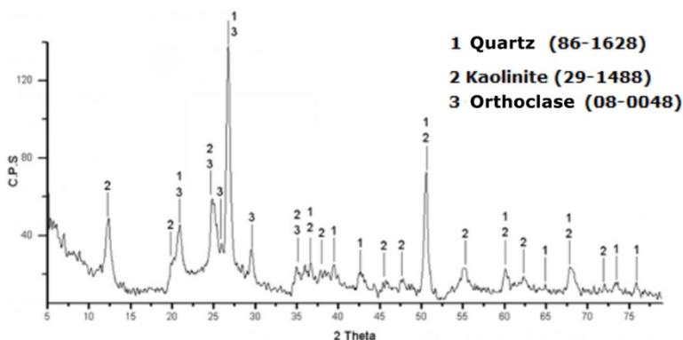
**Figure 2** –Diffractogram of the ceramic body.
