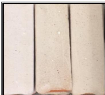
**Figure 9** – Samples fired at 850, 900 and 1000°C.
