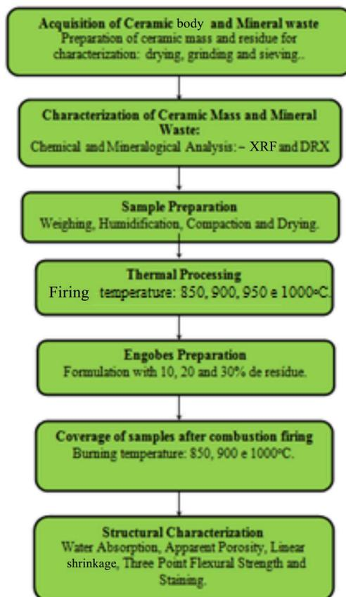
**Figure 1** – Simplified flow chart for the production of ceramic tiles.
