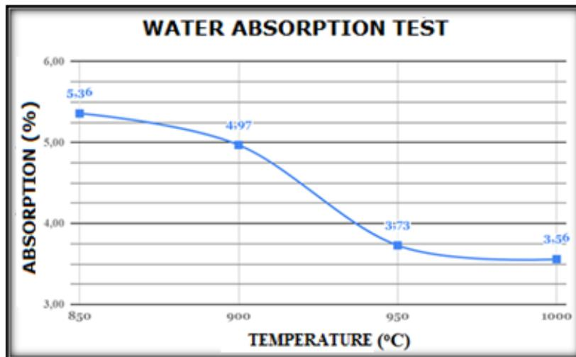
**Figure 5** – Water absorption graph of samples at different firing temperatures.
