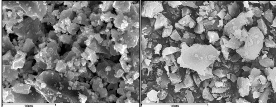
**Figure 1.** Micrographs of brick particles (L) and ceramic tile (B) particles
