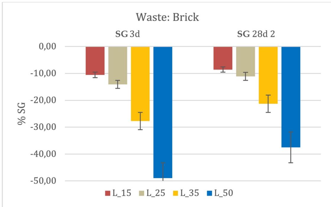
**Figure 6.** Strength gain in mortars with brick waste
