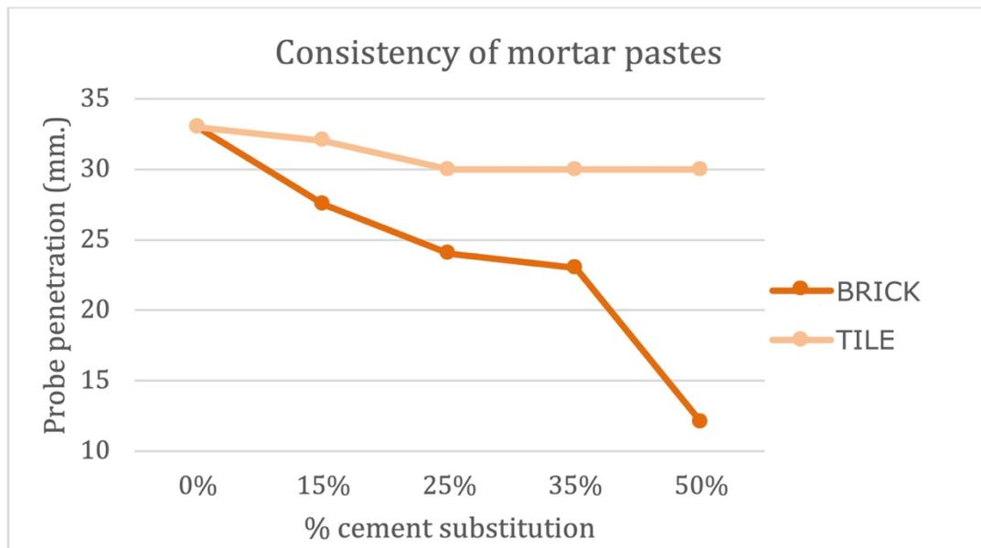
**Figure 2.** Consistency of pastes with cement replaced by waste
