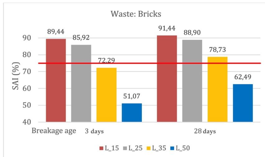
Figure 8. SAI (%) according to age and % brick substitution
