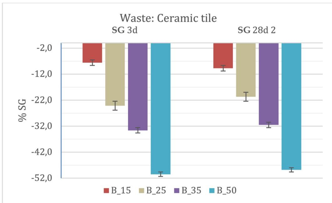
**Figure 7.** Strength gain in mortars with ceramic tile
