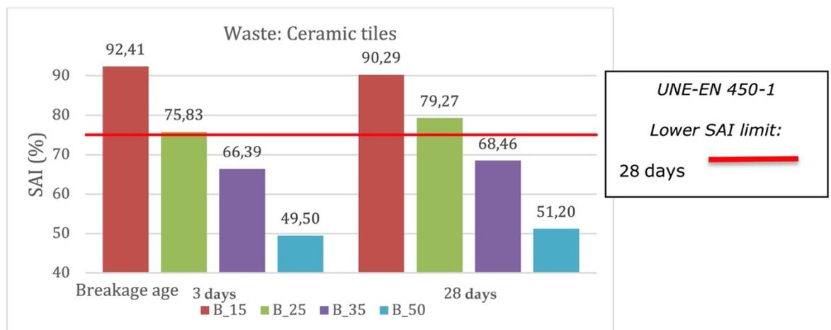
Figure 9. SAI (%) according to age and % ceramic tile substitution
