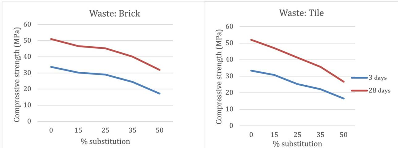
**Figures 4 and 5.** Compressive strength of mortars with brick and tile waste
