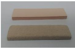
Ceramic pieces were successfully printed with this technology. However, work is ongoing to improve the printing composition in order to optimise different parameters such as green and fired mechanical strength.
