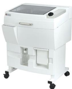
The first printing trials, using binder jetting technology, were performed using a Zcorp model 310 additive manufacturing printer.
