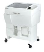
The first printing trials, using binder jetting technology, were performed using a Zcorp model 310 additive manufacturing printer.
