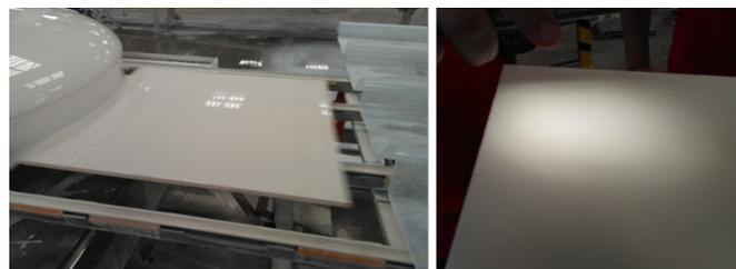
**Figure 4.** Glazing process and appearance of the glazed surface of a tile produced during the trial.
