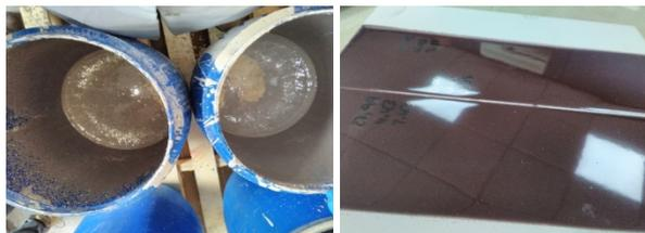
**Figure 5.** Comparison of the appearance of the (dispersed) slips and surfaces obtained using pigments made with and without treated quartz.
