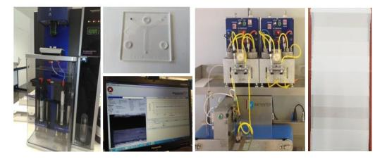
*Figure 1.* Optical rheometer for measuring viscosity at high shear rates (left). Ink-tester used in preparing the printing patterns of the developed digital inkjet formulations (right).
