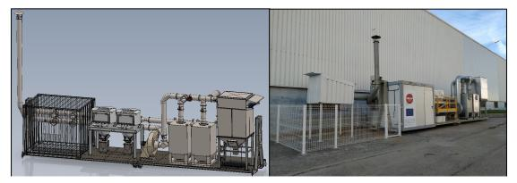
*Figure 2.* Detail of pilot plant design and its installation at the KERABEN Group facility (at Nules, Castellón province).
