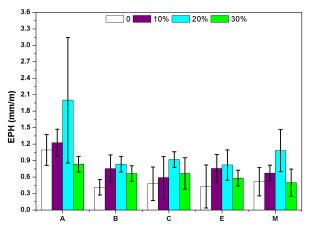
*Figure 3. Moisture expansion (EPM) of the sole clays and mixtures with dolomite addition after firing*
