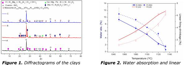
Figure 2. Water absorption and linear shrinkage of mixtures E and M
