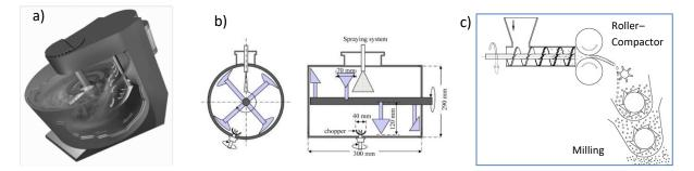
*Figure 1.* Images of the different technologies used for granulating materials: a) high-shear vertical granulator: b) low-shear horizontal granulator: and c) roller-compactor
