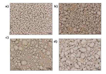
**Figure 2**. Image taken in a stereo microscope of the granules obtained by the different techniques compared in the study: a) spray-dried powder; b) material obtained in a high-shear vertical granulator; c) material obtained in a low-shear horizontal granulator; and d) material obtained with the roller–compactor technology
