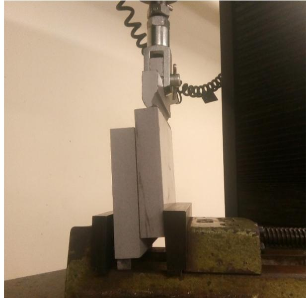
**Figure 1.** Assembled two-tile test specimen in the shear test stand of the universal testing machine.
