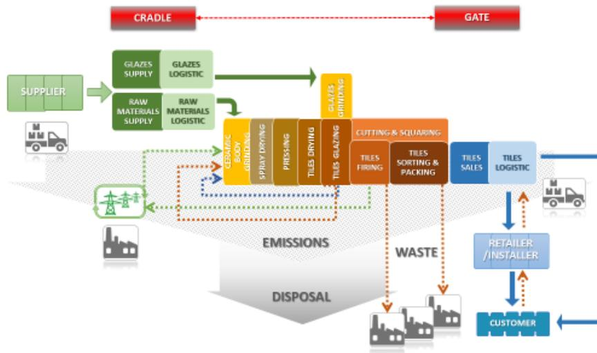
**Figure 1.** Ceramic production circular process flow.
