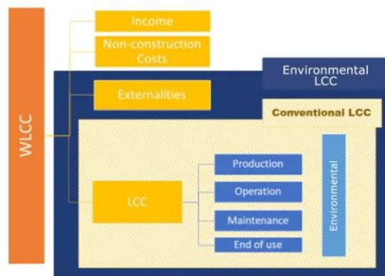
**Figure 2.** WLC and LCC elements (ISO 15686:5; 2017).
