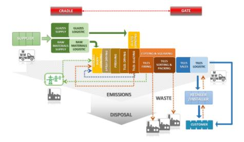
Figure 1. Ceramic production circular process flow.
