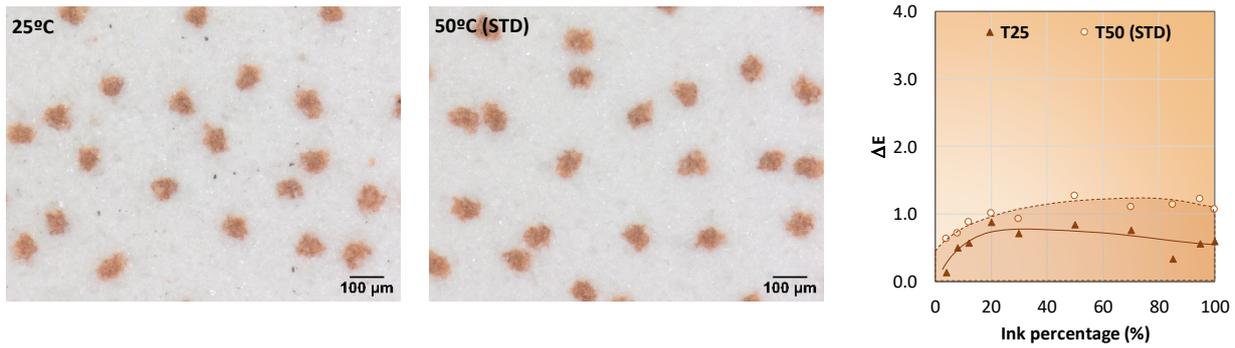
**Figure 6.** Influence of substrate temperature on unfired dot definition (left and centre) and on colour variation (right).
