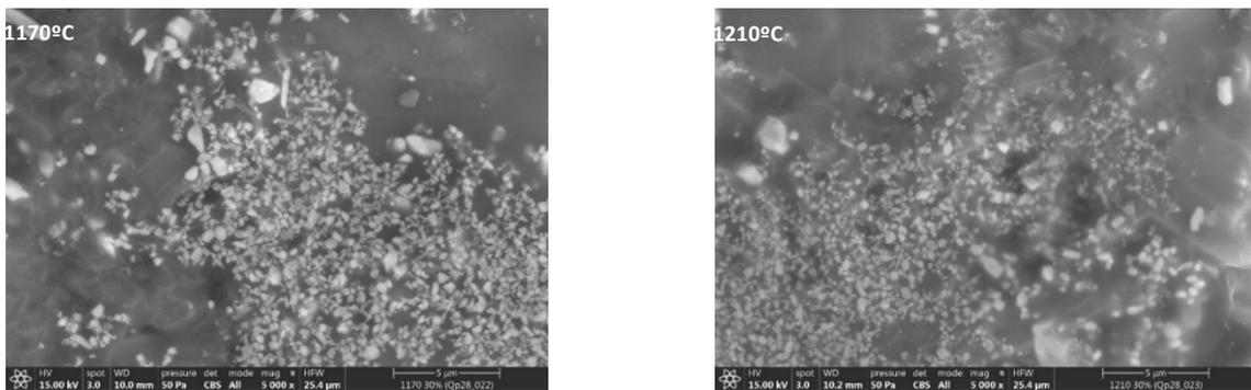
**Figure 12.** Surface viewed in the SEM of the patches printed with 30% ink. 1170°C (left) and 1210°C (right).
