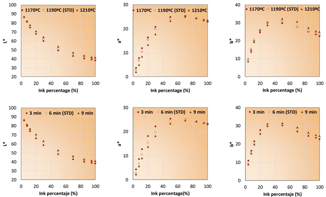
**Figure 10.** Influence of  $T_{max}$  (top) and  $t_p$  (bottom) on the chromatic coordinates.
