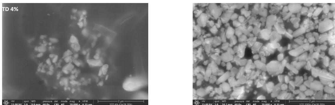
**Figure 5.** Surface viewed in the SEM of the patches printed with 4% (left) and 100% (right) ink under standard conditions (STD).
