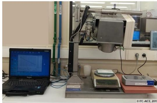
**Figure 2.** Set-up used to calibrate the infrared sensor.
