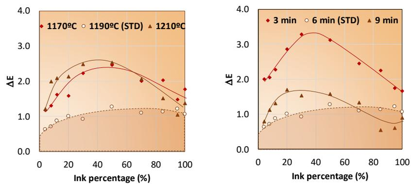
**Figure 13.** Influence of  $T_{max}$  (left) and  $t_p$  (right) on colour variation.
