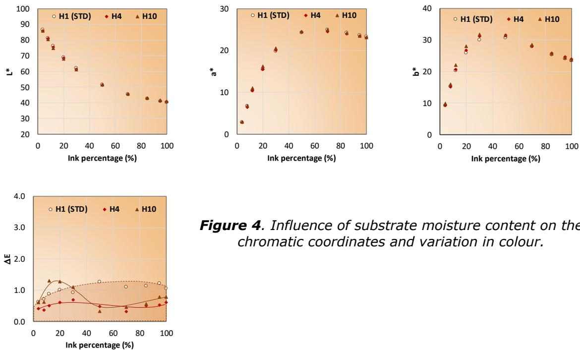
**Figure 4.** Influence of substrate moisture content on the chromatic coordinates and variation in colour.
