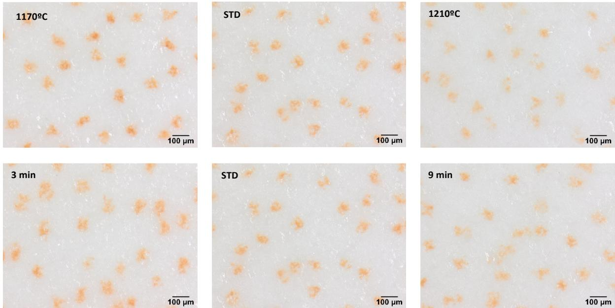
**Figure 11.** Influence of  $T_{max}$  (top) and  $t_p$  (bottom) on dot definition.
