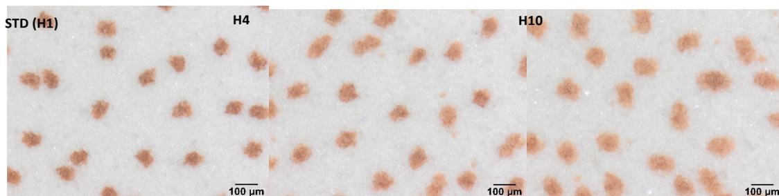
**Figure 3.** Influence of substrate moisture content on dot definition. Unfired piece.
