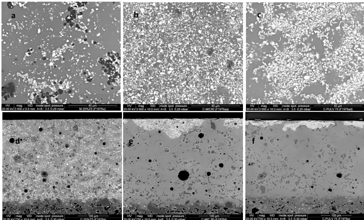
**Figure 4.** Appearance of the transparent glaze after mass addition of 20% zircon (a, d) and surface deposition of MIC-2 (b, e) and PULV-2 (c, f). The top images show the surface and the bottom images the cross-section.
