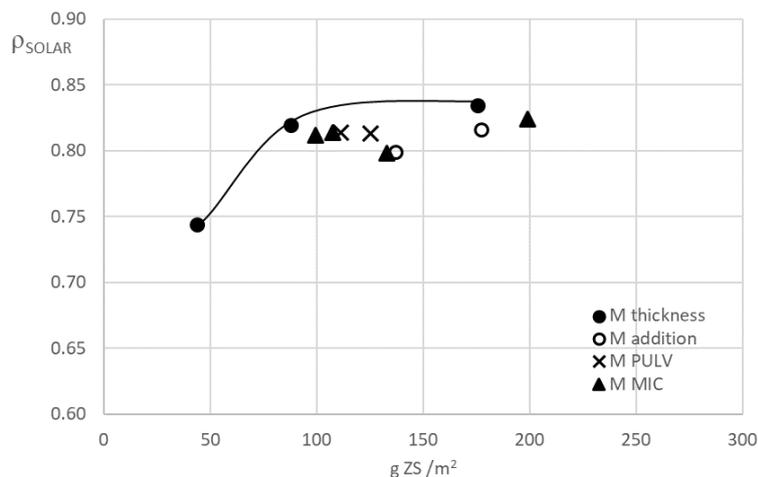
**Figure 3.** Reflectance of the matt glaze as a function of its zircon content (g/m<sup>2</sup>).
