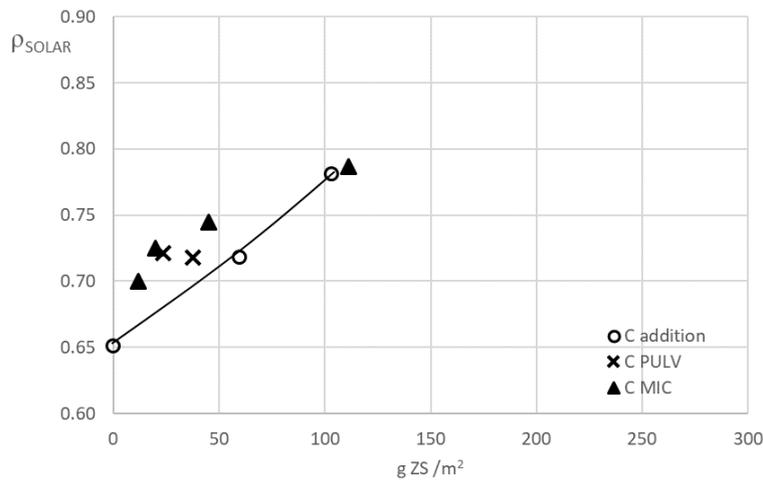
**Figure 2.** Reflectance of the transparent glaze as a function of its zircon content (g/m<sup>2</sup>).
