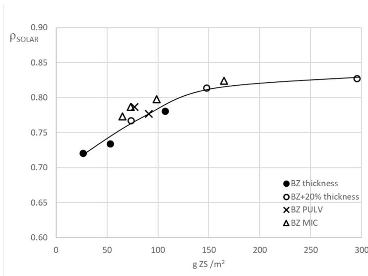
**Figure 1.** Reflectance of the zirconium white glaze as a function of its zircon content (g/m<sup>2</sup>).
