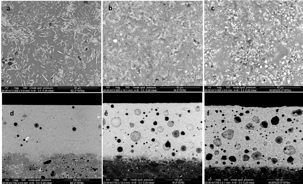
**Figure 5.** Surface and cross-section of the zirconium white glaze (a, d), matt glaze (b, e), and matt glaze with 20% ZS mass addition (c, f). The top images show the surface and the bottom images the cross-section.
