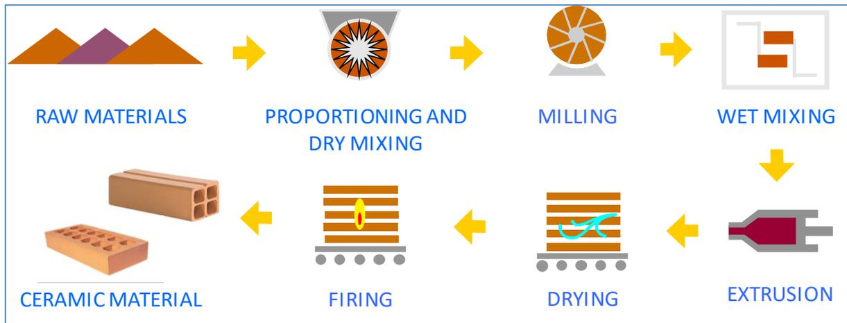
**Figure 1.** Process of obtaining ceramic material by extrusion
