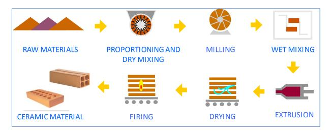
Figure 1. Process of obtaining ceramic material by extrusion
