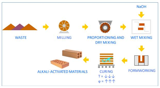
Figure 2. Process of obtaining alkali-activated material
