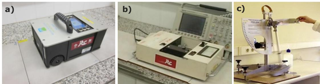
**Figure 1.** Devices used to determine slip resistance: a) BOT-3000E tribometer, b) Tortus® tribometer, and c) Friction pendulum.
