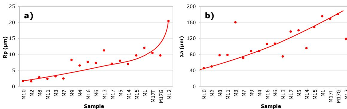
**Figure 9.** Variation of parameters: a) Rp and b) λa for the test samples according to the classification obtained.
