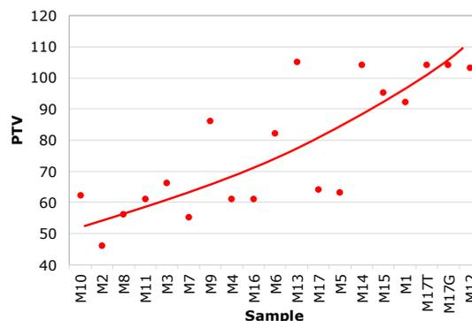
Figure 5. PTV determined with the friction pendulum.
