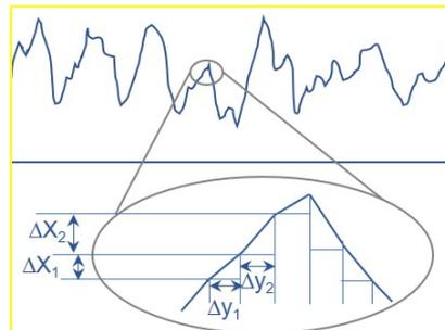
**Figure 10.** Obtainment of parameter  $\Delta_a$  from the roughness profile.
