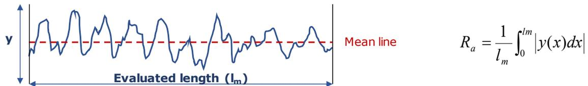
**Figure 8.** Obtainment of parameter Ra from the roughness profile.
