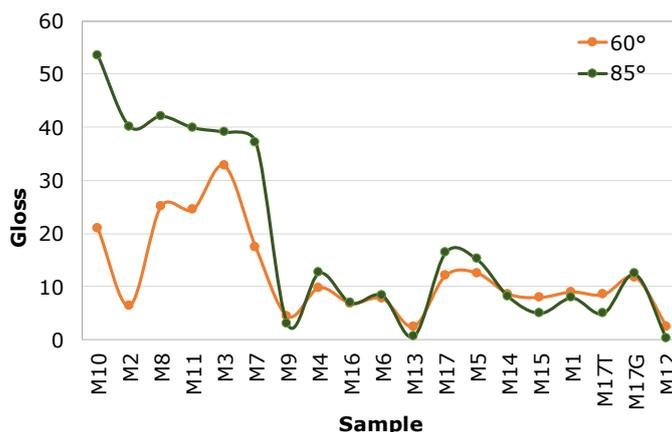
**Figure 2.** Gloss measured at 60 and 85° angles for all test pieces, ordered according to their tactile classification.
