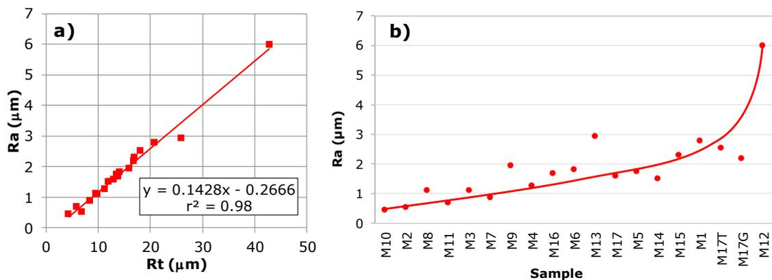
**Figure 7.** a) Relationship between roughness parameters Ra and Rt. b) Variation of parameter Ra for the test samples according to the classification.
