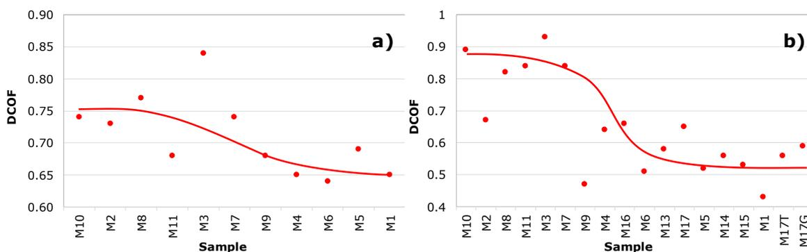
Figure 4. Dynamic coefficient of friction: a) BOT-3000E and b) TORTUS.
