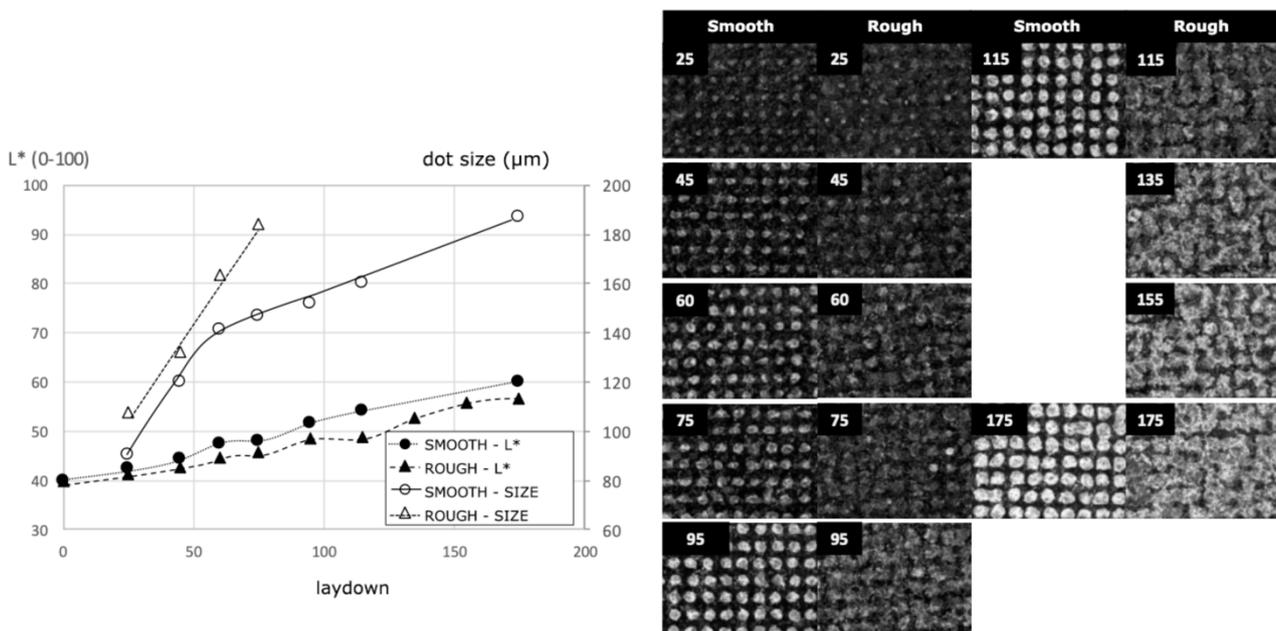
Figure 10. Comparison of lightness (L\*) and dot size of the 5% patch applied on the SMOOTH body and the ROUGH body at different laydowns.
