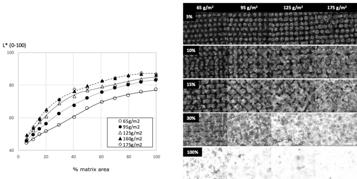
**Figure 5.** Ink NDS 30. Appearance of applied patches and L\* value on modifying application laydown.
