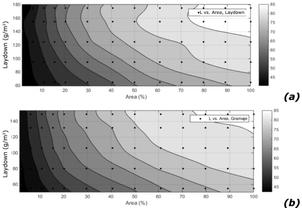
**Figure 7.** Lightness map as a function of applied laydown ( $W$ ) and % grey level ( $A$ ) of the patch, for inks NDS 30 and NDS 50.
