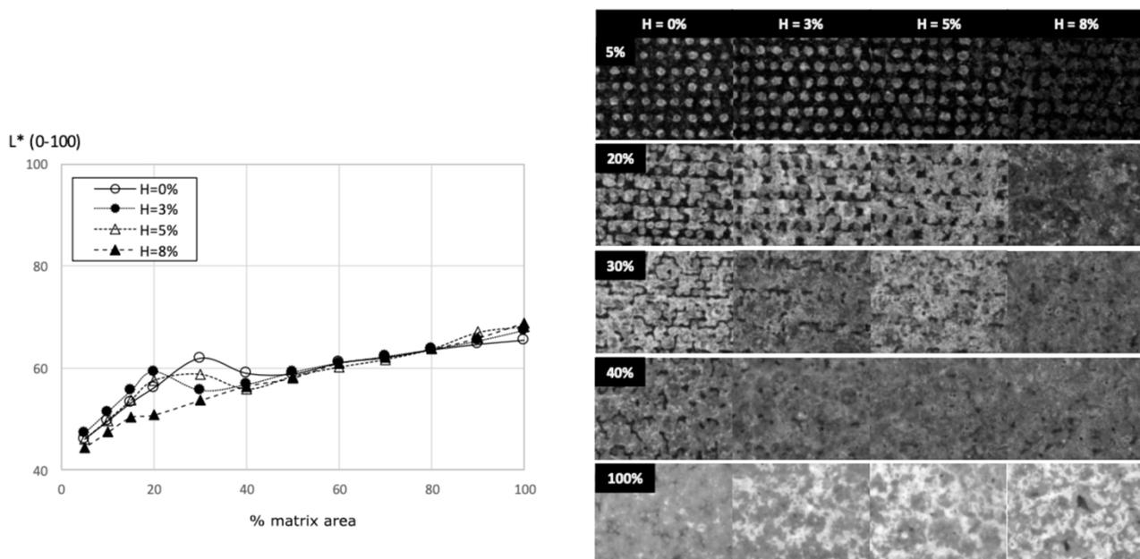
**Figure 8.** Effect of body moisture content on ink NDS 28 application. Laydown: 75 g/m<sup>2</sup>.
