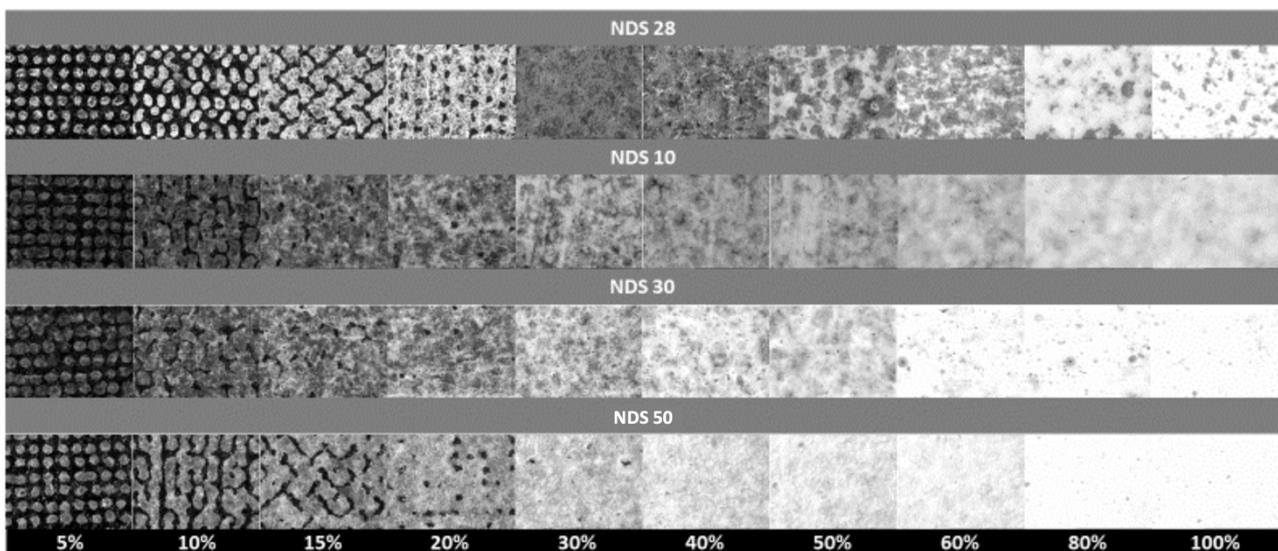
**Figure 4.** Appearance of the NDS 28, NDS 10, NDS 30, and NDS 50 ink applications, with the different Bayer 8x8 matrix grey levels and  $60\text{g}/\text{m}^2$  laydown (considering only the solids).
