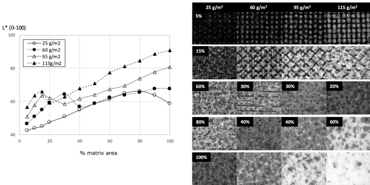
**Figure 6.** Ink NDS 28. Appearance of applied patches and L\* value on modifying application laydown.
