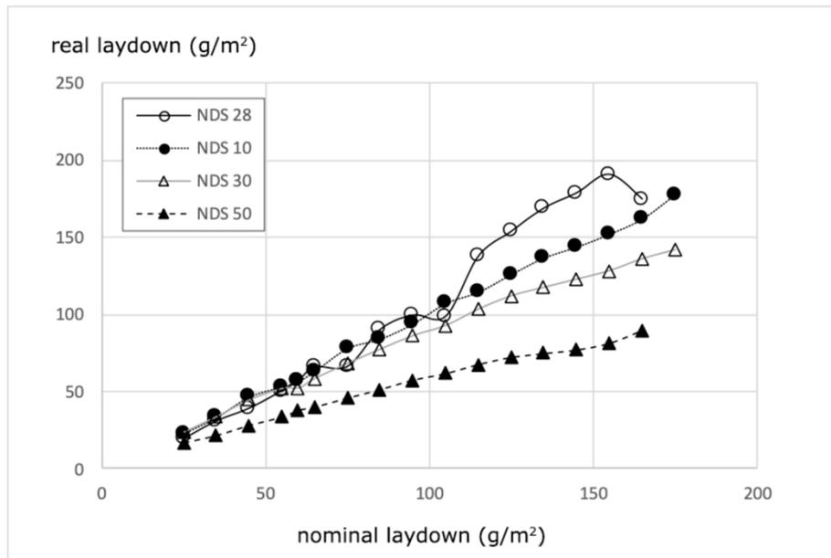
Figure 2. Calibration of the real g/m<sup>2</sup> laydown, using the waveform developed for each ink.
