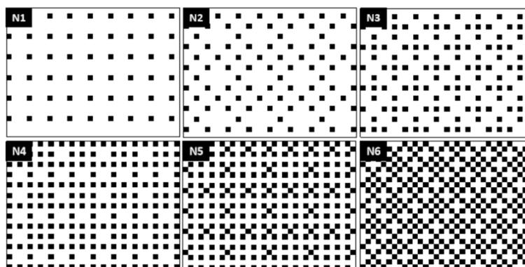
**Figure 1.** Layout of the dots applied in the first six levels of grey of the Bayer 8x8 matrix.
