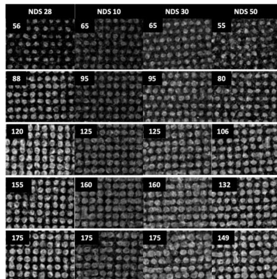
Figure 3. Size and distribution of the dots obtained with the four inks applied with the 5% matrix at different g/m<sup>2</sup> laydowns, indicated on the label of each image.
