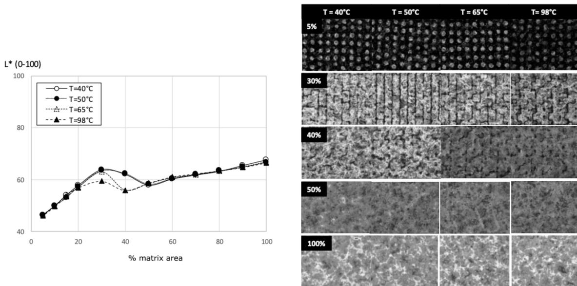
Figure 9. Effect of body temperature on ink NDS 28. Laydown: 75 g/m<sup>2</sup>.
