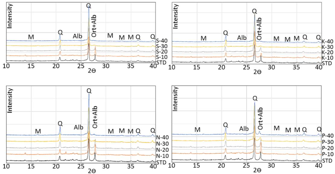
**Figure 2.** Fired XRD patterns and mineral phases determined of the recipes and standard body.
