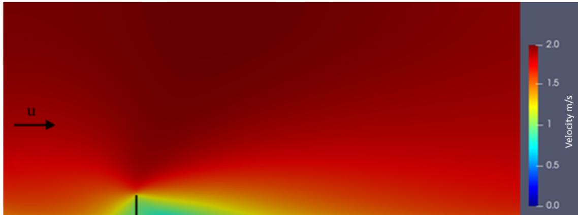
**Figure 2.** Wind profile in a scenario with a 12m high porous perimeter screen.
