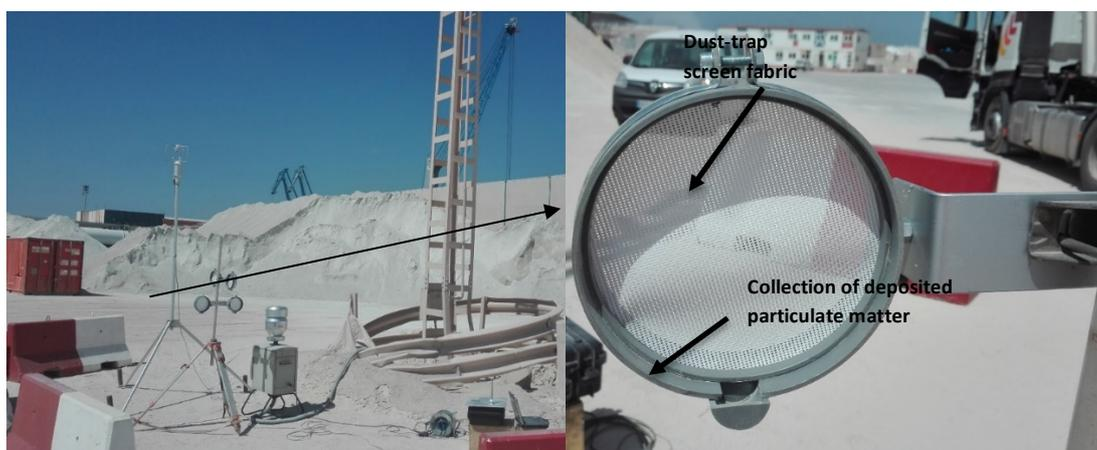
**Figure 4.** Experiment set-up on the Transversal pier at the Port of Castellón.
