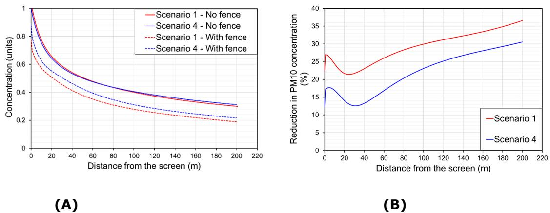
**Figure 7. (A):** Variation in PM10 concentration at a height of 5m downwind from the screen in scenarios 1 and 4 with and without a screen. **(B):** Reduction in PM10 concentration in the same scenarios when the screen was present.
