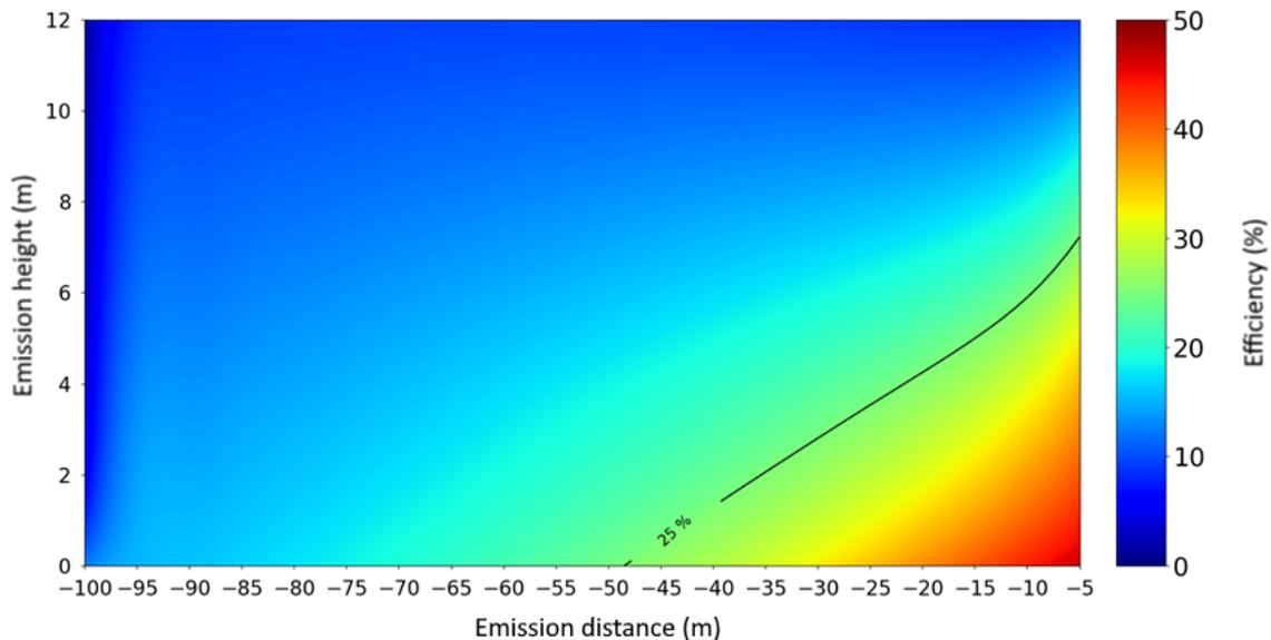
**Figure 5.** Screen efficiency map in scenario 1, according to emission point position.
