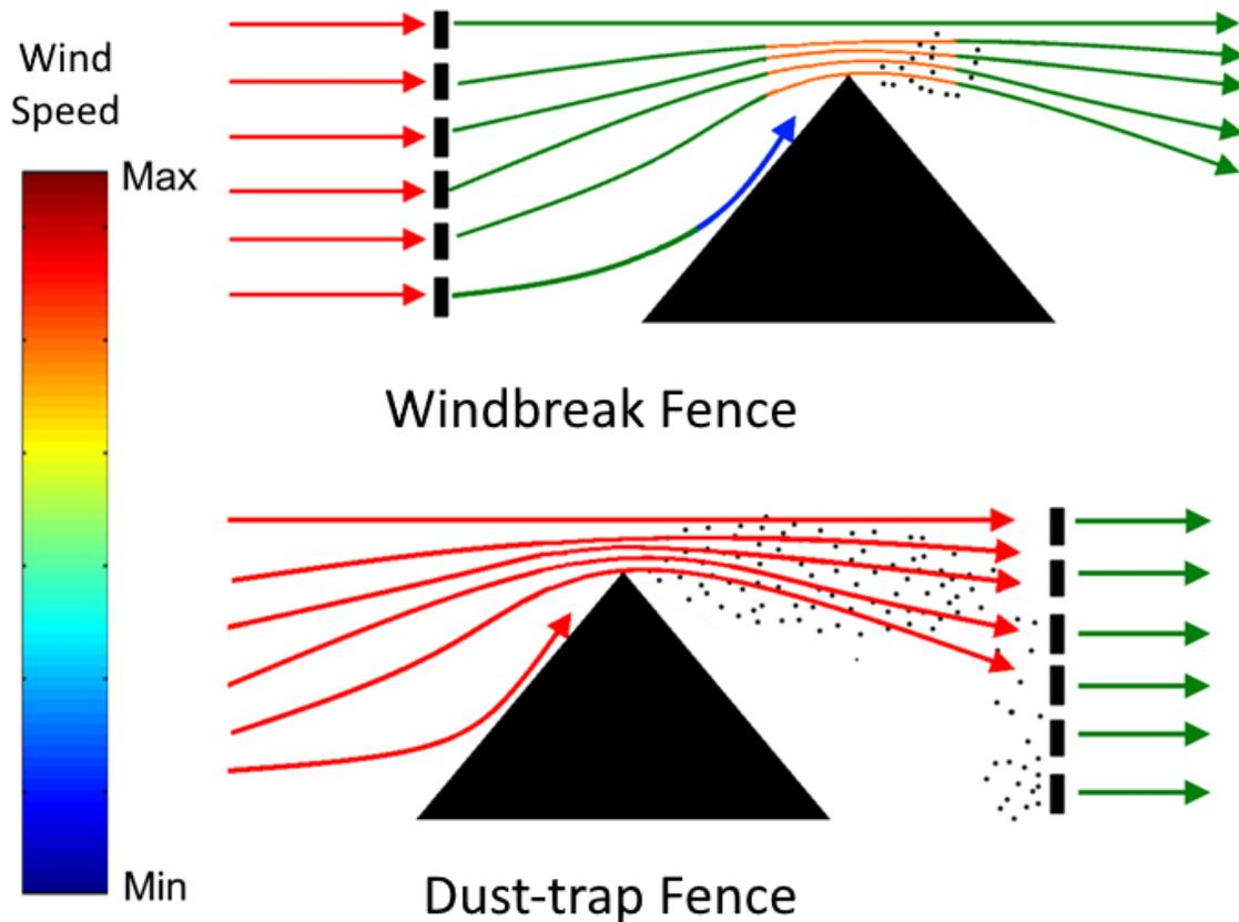
**Figure 1.** Effect of a porous screen on a stockpile of bulk material.
