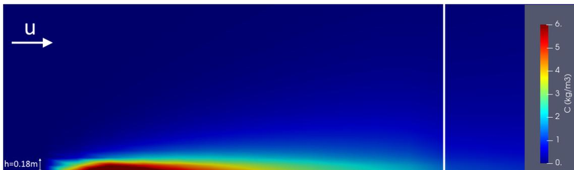
**Figure 3.** Concentration profile in a scenario with a 12m high porous perimeter screen.
